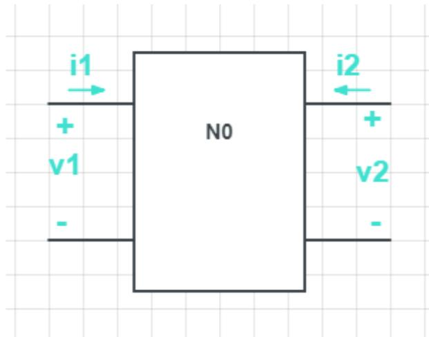
First we choose  $V_1, V_2$  as inputs and  $I_1, I_2$  as outputs and set  $\begin{bmatrix} I_1 \\ I_2 \end{bmatrix} = \begin{bmatrix} y_{11} & y_{12} \\ y_{21} & y_{22} \end{bmatrix} \begin{bmatrix} V_1 \\ V_2 \end{bmatrix}$
