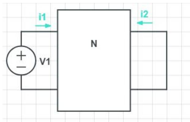
$$y_{11} = \frac{I_1}{V_1} \Big|_{V_2=0}$$
