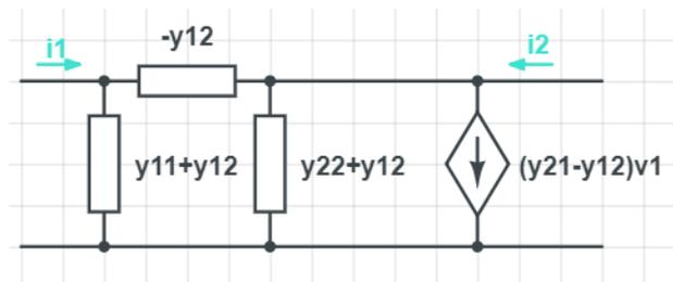
Find the y parameters and represent the following circuit in this equivalent form.
