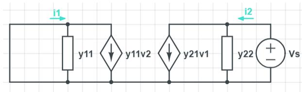
If  $y_{12} = y_{21}$ ;  $i_1 = i_2$ . Can interchange the position of the voltage source and the point at which current is measured.
