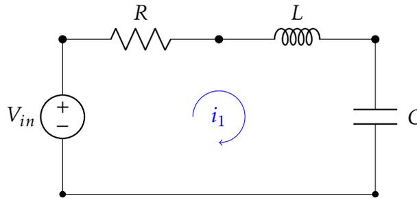
$$V_{in} = iR + L \frac{di}{dt} + \frac{1}{C} \int i dt$$
