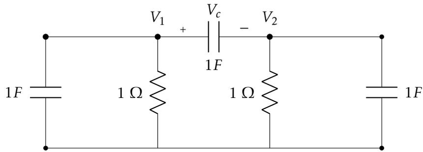
$$\underbrace{\begin{bmatrix} 2s+1 & -s \\ -s & 2s+1 \end{bmatrix}}_{\text{Node basis Network matrix (admittance matrix)}} \begin{bmatrix} V_1 \\ V_2 \end{bmatrix} = \begin{bmatrix} a \\ b \end{bmatrix}$$
