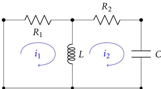
$$\underbrace{\begin{bmatrix} R_1 + sL & -sL \\ -sL & R_2 + sL + 1/sC \end{bmatrix}}_{\text{Network matrix (mesh basis)}} \underbrace{\begin{bmatrix} I_1 \\ I_2 \end{bmatrix}}_{\text{initial conditions}} = \underbrace{\begin{bmatrix} a \\ b \end{bmatrix}}_{\text{initial conditions}}$$
