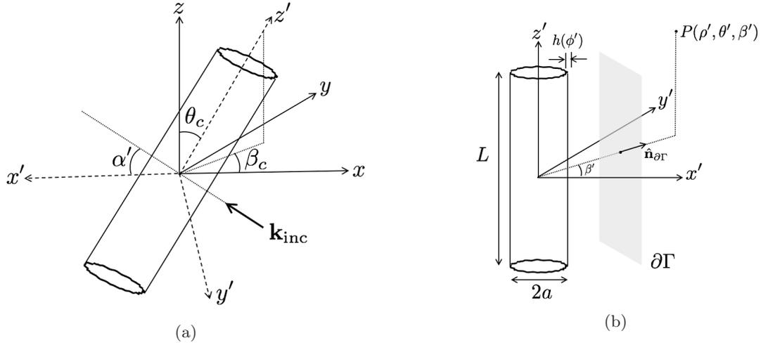
Figure 1: Schematic of the scatterer geometry. (a) shows the orientation of the coordinate systems used in the paper and (b) shows the effective surface  $\partial\Gamma$  used for computing the electromagnetic far field at point  $P$  for a finite cylinder.
