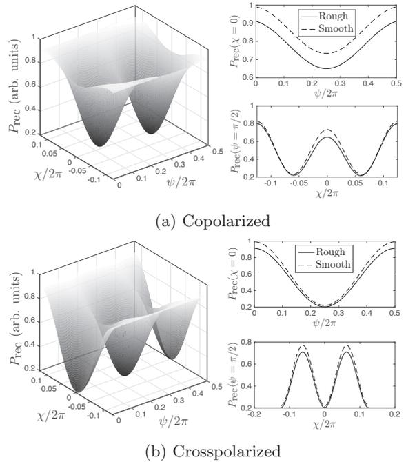
Figure 2: Variation of received power  $P_{\text{rec}}$  (arbitrary units) with the transmitting antenna orientation  $\psi$  and ellipticity  $\chi$ . In all simulations,  $a = 50$  cm,  $L = 100$  cm,  $\lambda_0 = 23$  cm,  $N = 10$  and cylinder dielectric constant  $\epsilon_r = 20 + 7.0j$ .
