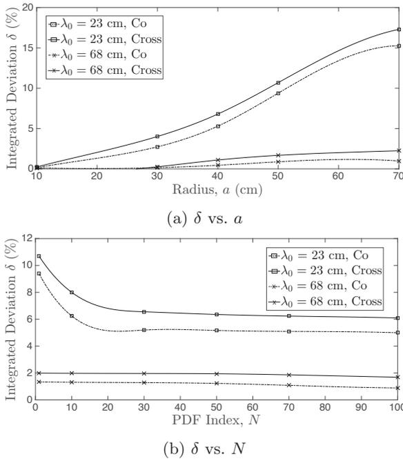
Figure 3: Variation of integrated deviation with cylinder radius  $a$  and the index  $N$ .  $L = 100$  cm and cylinder dielectric constant  $\epsilon_r = 20 + 7.0j$  is assumed in all the simulations,  $N = 1$  in (a) and  $a = 50$  cm in (b).
