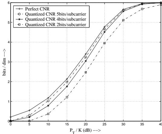
Figure 3: Performance of System 1 for various number of quantization levels. Target BER =  $10^{-5}$ . Constellations used QPSK, 16QAM, 64QAM.
