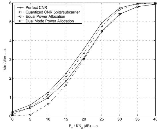
Figure 5: Performance comparison of System 1 and System 2. Constellations used with rates varying from 1 to 6. Notice the decreased performance gap between the different schemes.
