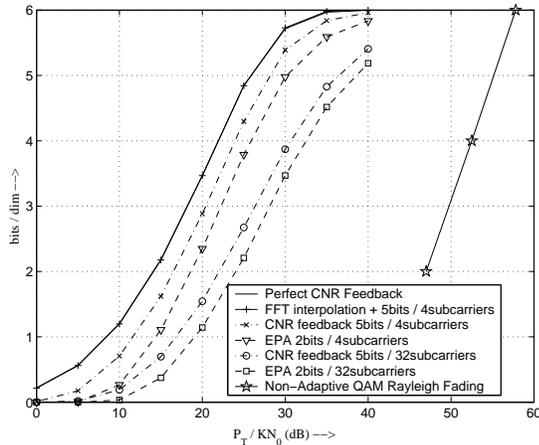
Figure 6: Spectral efficiency comparison for different grouping methods for group sizes 4, 32.
