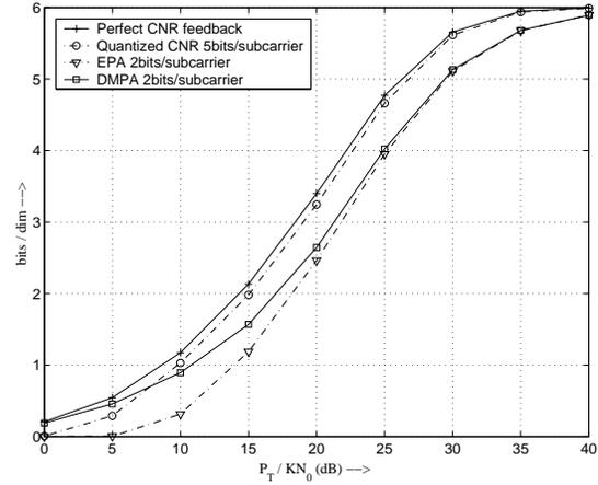
Figure 4: Performance comparison of System 1 and System 2. Constellations used QPSK, 16QAM, 64QAM.
