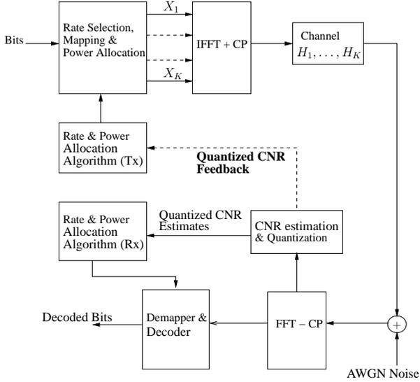
Figure 1: Same allocation algorithms performed at transmitter and receiver, and quantized CNR values fed back from receiver to transmitter.
