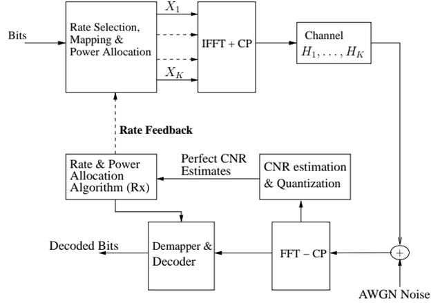
Figure 2: Allocation algorithm performed only at receiver, and rate allocation fed back to transmitter.
