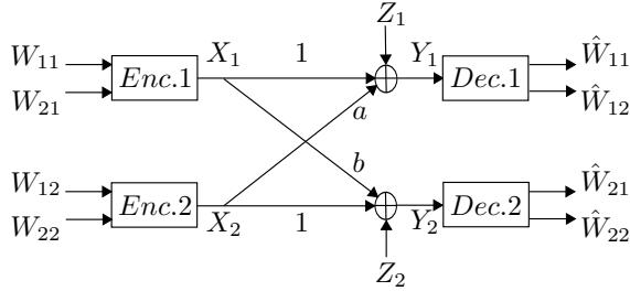
Fig. 1. Two user scalar Gaussian X channel
