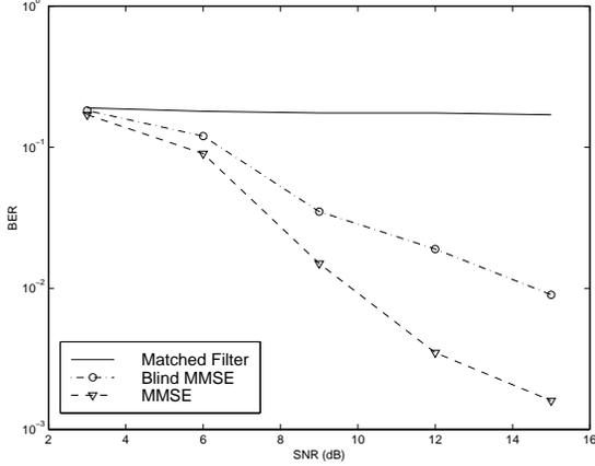
Fig. 1. Performance comparison of blind MMSE and conventional MMSE receivers – number of users = 24, all users have equal power
