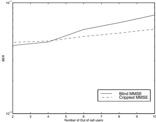
Fig. 2. Performance of Blind MMSE and Crippled MMSE receivers – number of in-cell users = 10, all users have equal power
