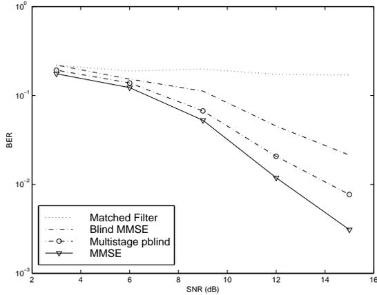
Fig. 5. Performance of partially blind multiuser detector based on soft-decision feedback – number of in-cell users = 12, number of out-of-cell users = 12, users within cell have power between 0 and 6 dB higher than the user-of-concern, power of out-of-cell users = 36% of power of in-cell users.
