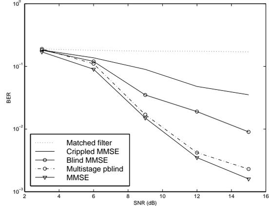
Fig. 4. Performance of partially blind multiuser detector based on soft-decision feedback – number of in-cell users = 12, number of out-of-cell users = 12, users within cell have equal power, power of out-of-cell users = 36% of power of in-cell users.
