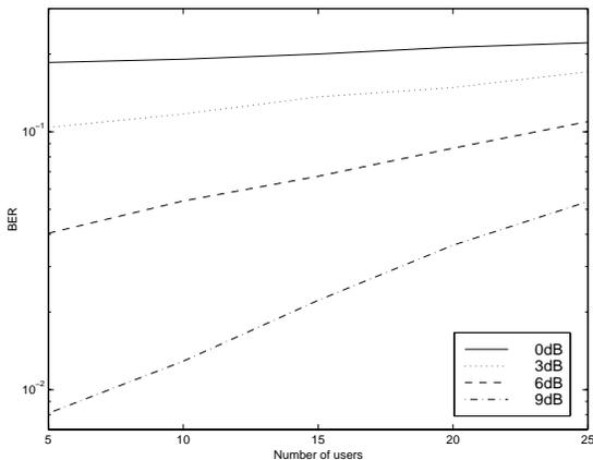
Fig. 3. Sensitivity of blind MMSE algorithm to background interference, all users have equal power.
