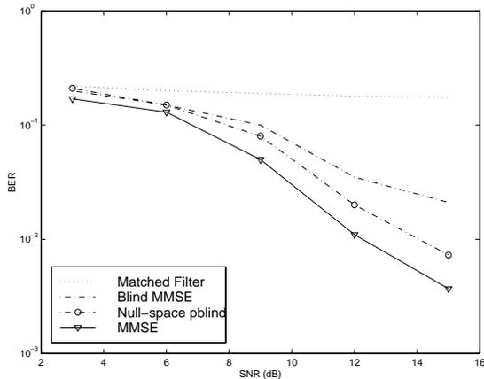
Fig. 6. Performance of null-space based partially blind multiuser detector – number of in-cell users = 12, number of out-of-cell users = 12, users within cell have power between 0 and 6 dB higher than the user-of-concern, power of out-of-cell users = 36% of power of in-cell users.
