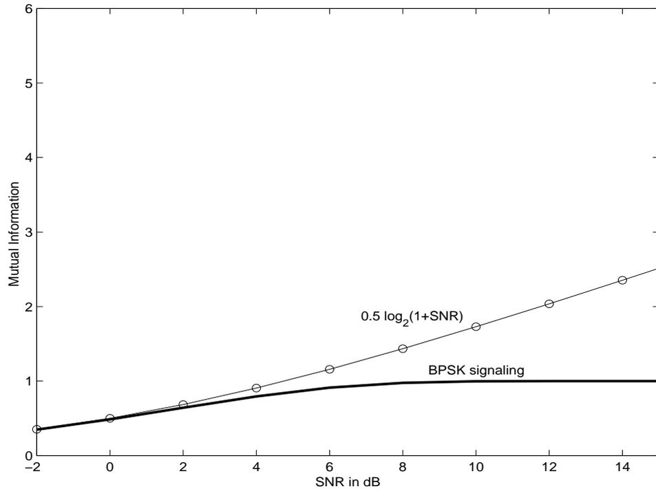
Figure 2: Mutual Information for BPSK signaling vs. SNR
