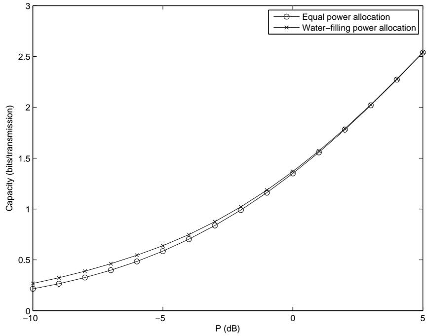
Figure 1: Comparison of capacities with equal power allocation and water-filling power allocation
