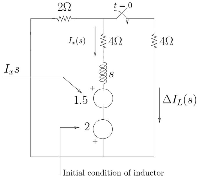
Figure 9: (*Problem 3*) Incremental network in the Laplace domain
