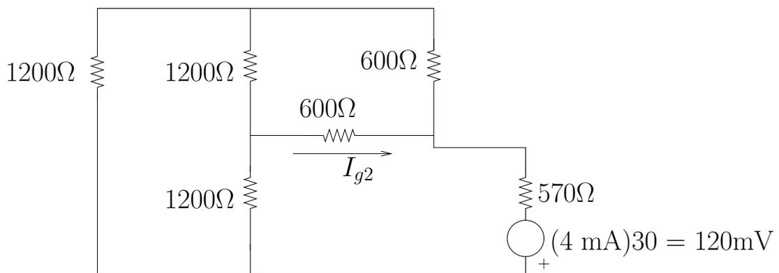
Figure 7: (*Problem 2*) Incremental network for  $R_x = 570\Omega$
