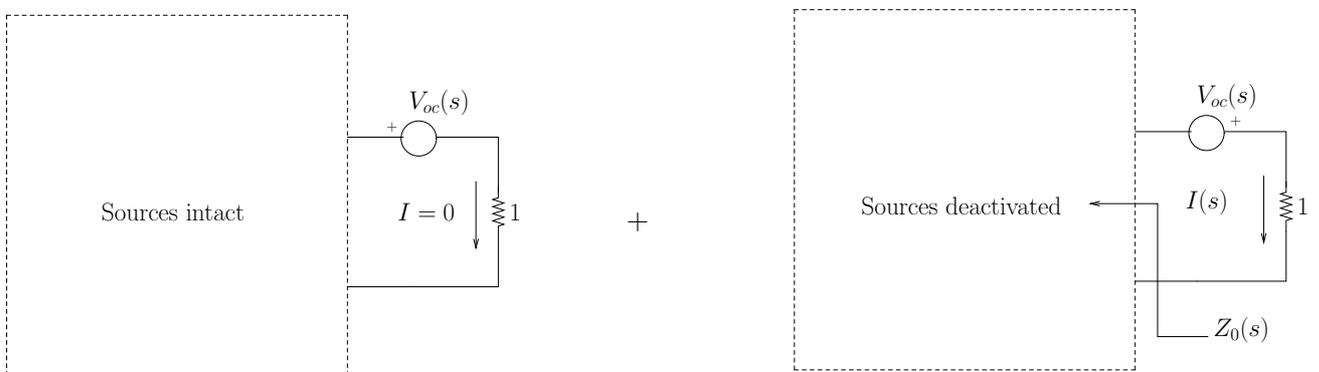
Figure 5: (*Problem 1(b)*) Applying the superposition principle
