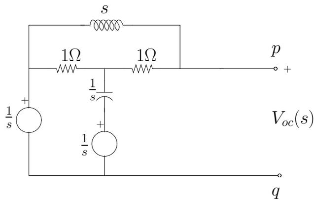
Figure 1: (*Problem 1(a)*) Laplace-transformed network
