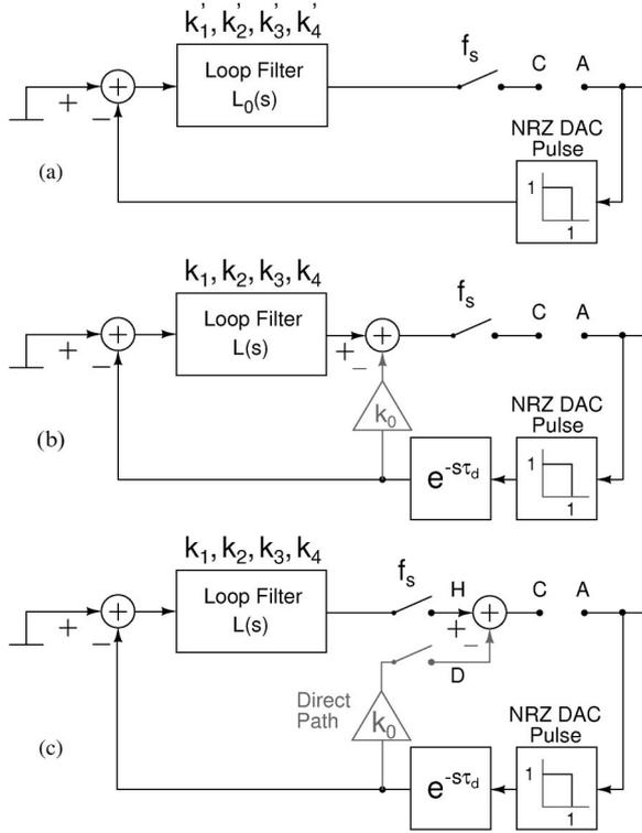
Fig. 2.  $\Delta\Sigma$  modulator loop broken at the quantizer. (a) Ideal (no ELD). (b) With ELD, the discrete-time loop filter response from A to C is adjusted to be the same as in the ideal case. (c) Fig. 2(b) modified to show the sampled outputs of the loop filter and the direct path separately.
