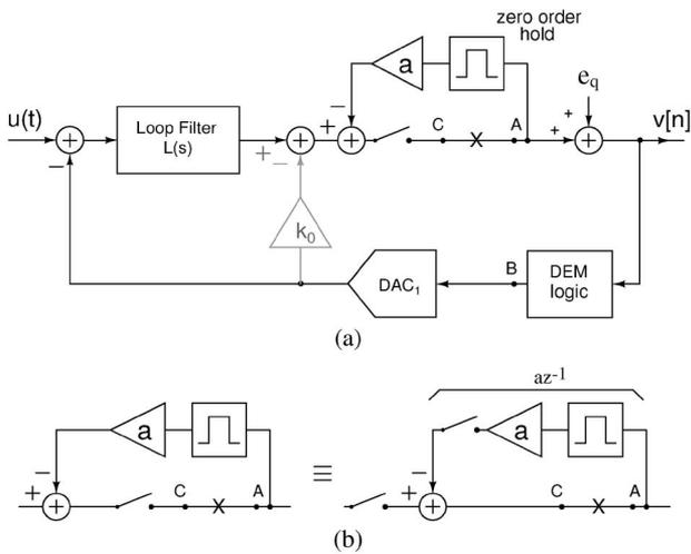
Fig. 5. (a)  $\Delta\Sigma$  modulator with additive quantization noise  $e_q$  and (b) calculating the transfer function of the fast loop.
