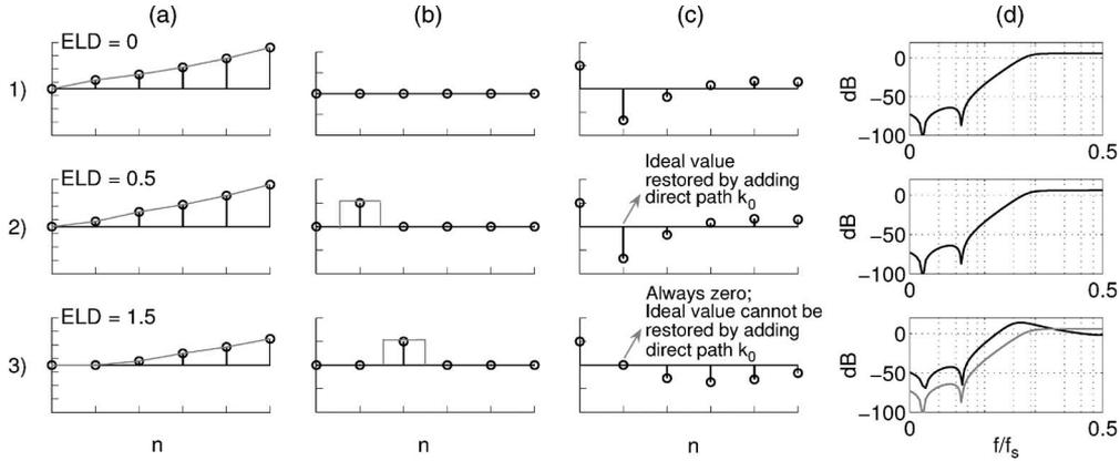
Fig. 3. Limitation of conventional ELD compensation with  $\tau_d > 1$ . Each row shows the discrete-time equivalent impulse response of the loop filter  $L(s)$ , the direct path  $k_0$  (with the continuous-time waveforms in gray), and the NTF impulse response that results from the combination. For  $ELD > 1$ , the second sample of the NTF is always zero and results in a poor NTF. The sampling rate is 1 Hz. For clarity, columns (a)–(c) are shown to different scales.
