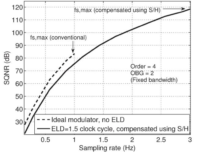
Fig. 8. Variation of SQNR with sampling frequency ( $f_s$ ).  $f_s$  is normalized to the  $f_{s,\text{max}}$  of the conventionally compensated modulator. The signal bandwidth is 1/50.
