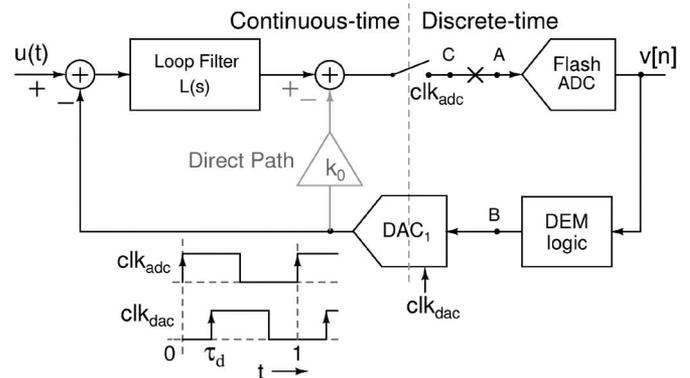
Fig. 1. Block diagram of a Cascaded Integrator with FeedForward summation (CIFF) CTDSM.  $k_0$  is the gain of the direct path required to compensate for ELD.
