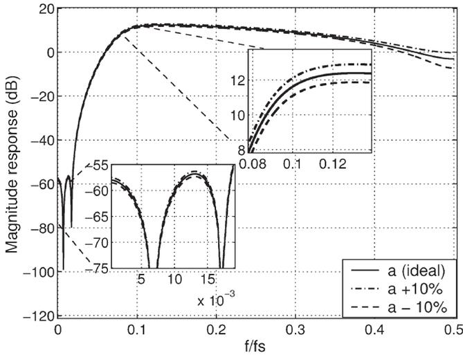
Fig. 10. Magnitude response of NTF for different values of gain coefficient  $a$ .
