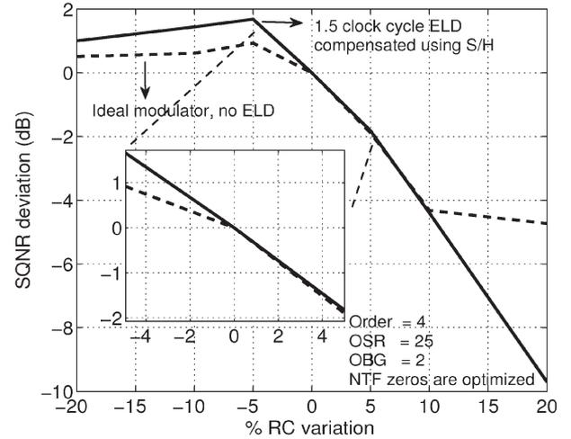
Fig. 9. Peak SQNR deviation from its ideal value versus time constant variations of the loop filter.
