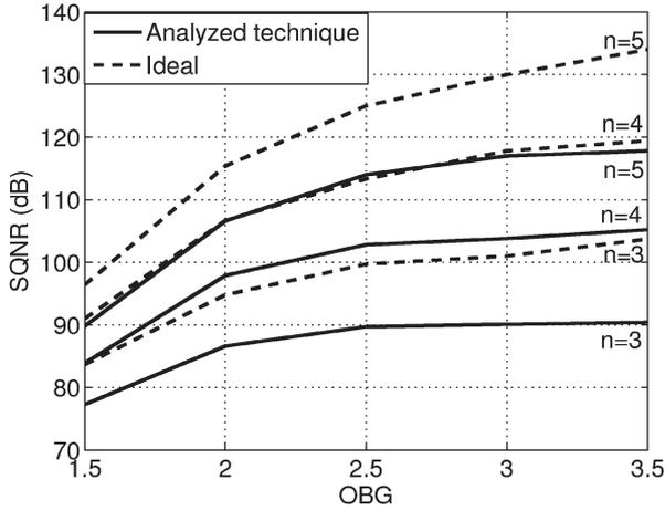
Fig. 7. Peak SQNR versus OBG for various orders. An ELD = 1.5 is compensated using the proposed technique. A 4-bit quantizer is assumed (OSR = 25).
