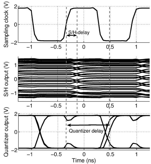
Fig. 12. Eye diagram of the S/H and the quantizer output. Time period = 1.25 ns.
