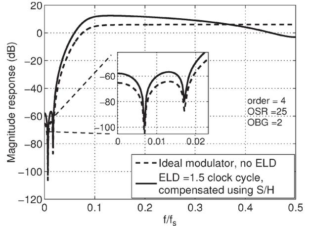
Fig. 6.  $|NTF|$  showing the effect of  $(1 + az^{-1})$  in the analyzed modulator.
