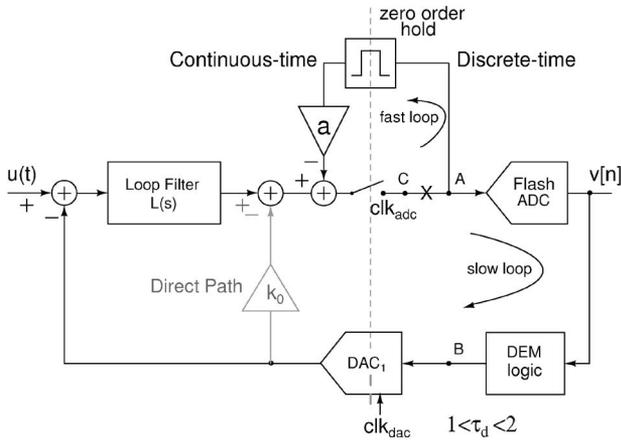
Fig. 4. Block diagram of a  $\Delta\Sigma$  ADC with ELD compensation obtained by bypassing the flash ADC using an S/H.
