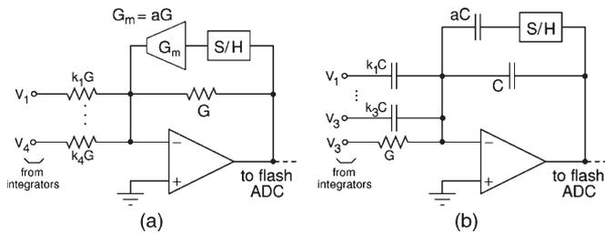
Fig. 11. Implementation of the fast loop with (a) a loop filter with a separate summing amplifier and (b) a loop filter with the last integrator used for summation.
