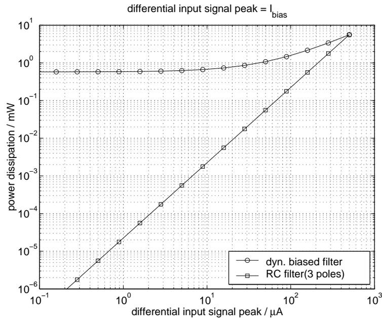
Figure 7.21: Power dissipation versus the input signal: Pseudo-differential ladder filter (Fig. 7.18(a)) and passive RC filter (Fig. 7.18(c)).
