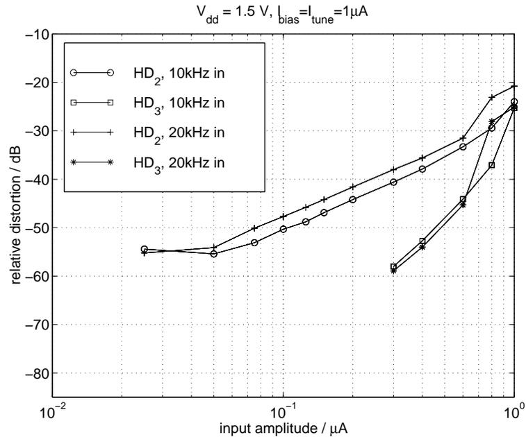
Figure 8.36: Distortion performance of the filter with  $1 \mu\text{A}$  bias current.
