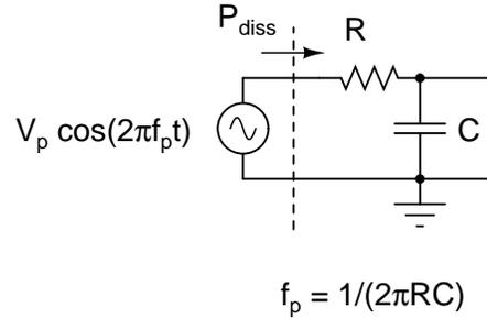
Figure 2.1: Sinusoidal source driving a first-order RC filter.
