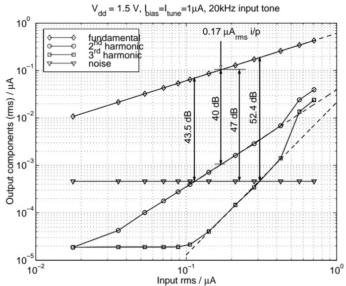
Figure 8.38: Signal, noise and distortion in the second order filter with  $1\mu\text{A}$  bias current.
