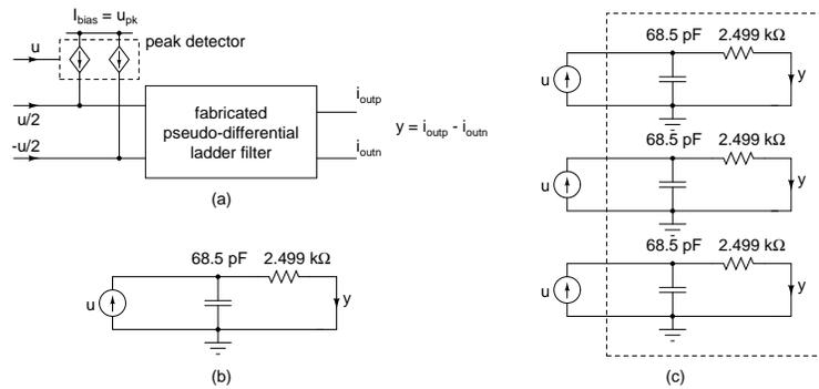
Figure 8.14: (a) Pseudo differential filter biased from an ideal peak detector, (b) Current mode RC filter with  $S/N = 53.7$  dB for a  $3 \mu A$  peak input, (c) Three first-order RC filters.
