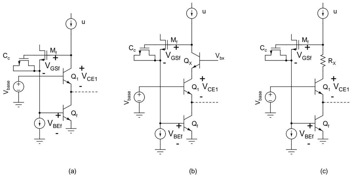
Figure 8.41: (a) Feedback used to establish the collector currents, (b) Cascoding to maintain a constant collector-emitter voltage of  $Q_1$ , (c) Using a resistor to minimize the variations in the collector-emitter voltage of  $Q_1$ .
