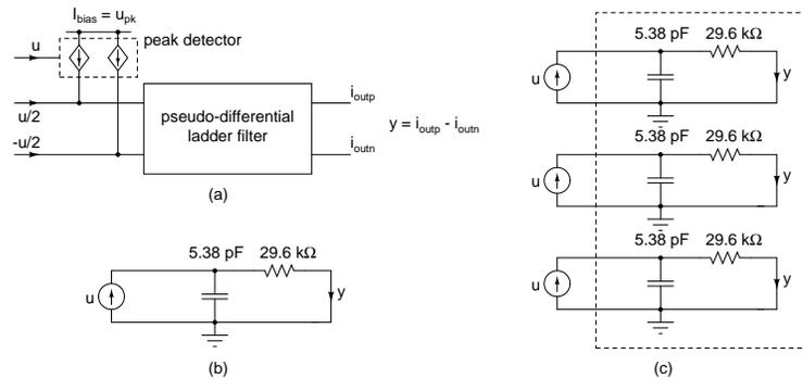
Figure 7.18: (a) Pseudo differential filter biased from an ideal peak detector, (b) Current mode RC filter with  $S/N = 48.5$  dB for a  $0.5 \mu\text{A}$  peak input, (c) Three first-order RC filters.
