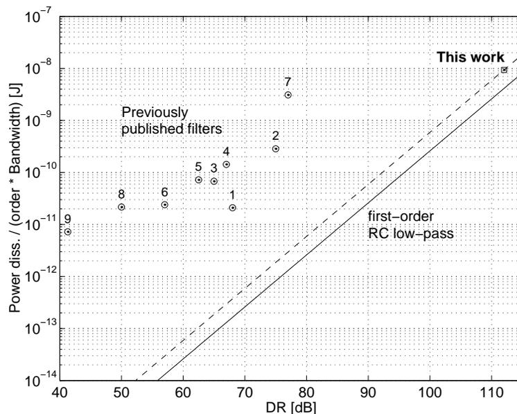
Figure 8.17: Power dissipation per pole and edge frequency vs. dynamic range
