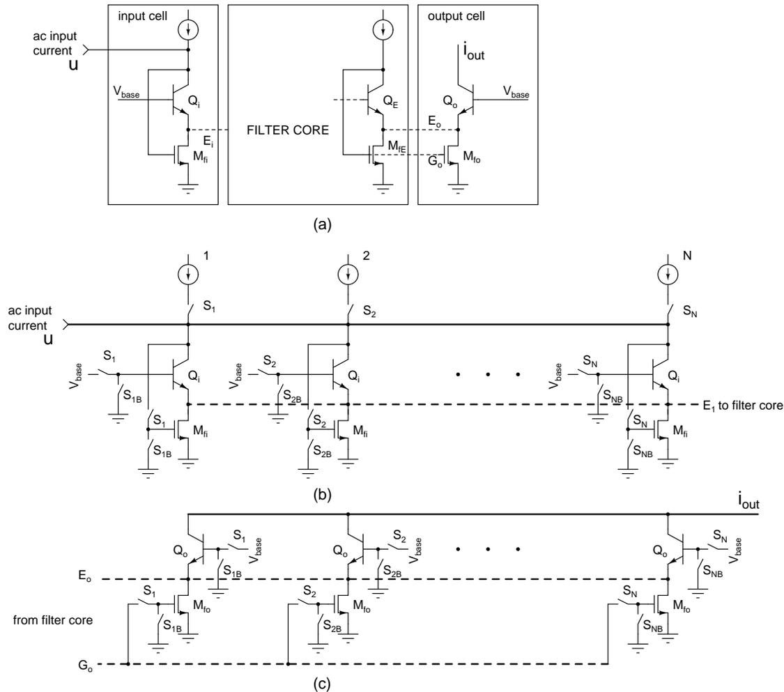
Figure 8.43: (a) Log-domain filter drawn in a general form, (b) Array of switched input cells, (c) Array of switched output cells.
