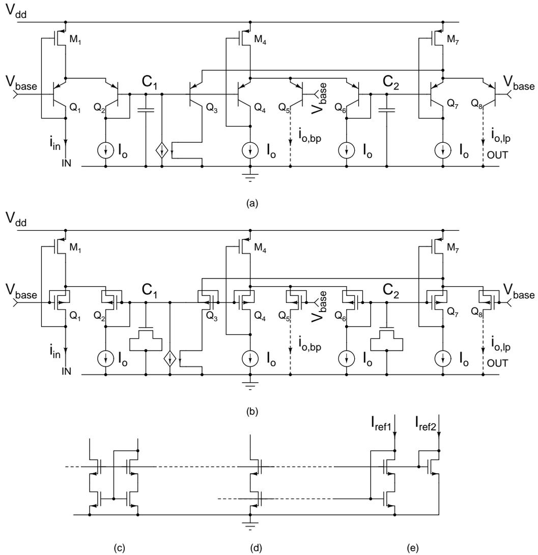
Figure 7.47: CMOS Log-domain realization of Fig. 7.46: (a) Log-domain topology, (b) Circuit in (a) redrawn with lateral PNP transistors (pMOS transistors with gate and bulk tied together) and MOS capacitors, (c) Current mirror, (d) Current source, (e) Bias generator.
