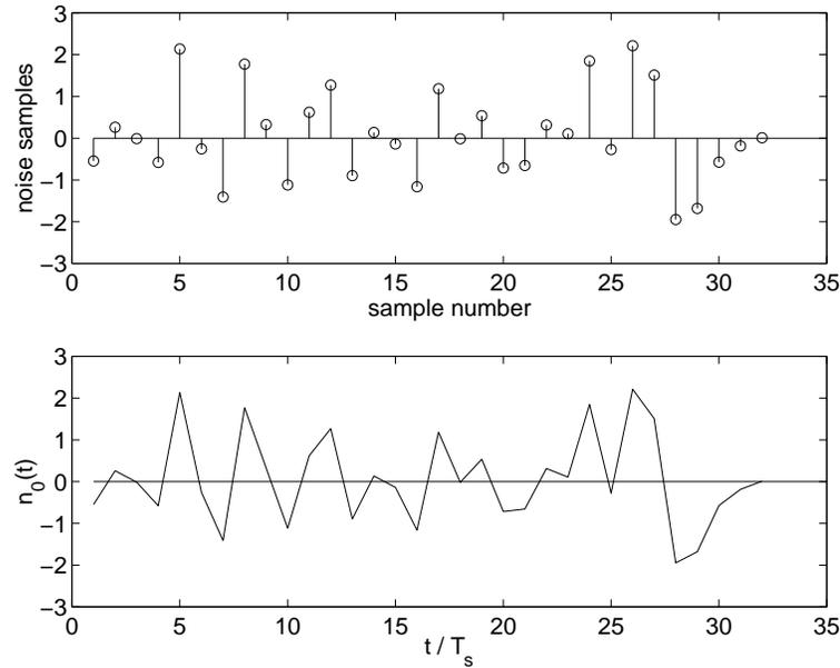
Figure 6.15: (a) Discrete time random sequence, (b) Linearly interpolated continuous time waveform.
