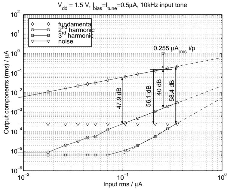
Figure 8.37: Signal, noise and distortion in the second order filter with  $0.5\mu\text{A}$  bias current.
