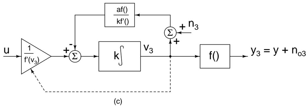
Figure 6.2: (a) Noise added at the input of the output nonlinearity, (b) Noise added after the input amplifier, (c) Noise added in the feedback path.
