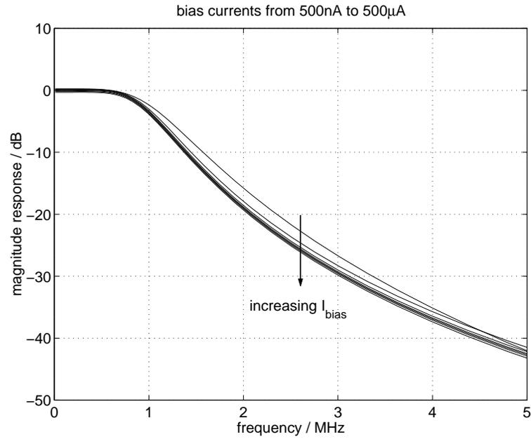
Figure 7.12: Frequency response with the bias current varied from 500 nA to 500  $\mu$ A.
