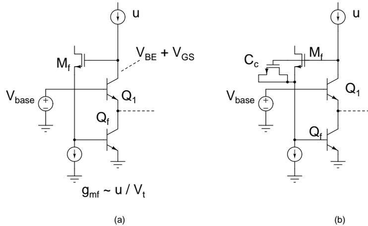
Figure 7.6: (a) Proposed feedback circuit for establishing collector currents in Fig. 7.3(c), (b) With frequency compensation.
