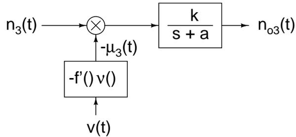
Figure 6.7: Noise equivalent circuit for Fig. 6.2(c).
