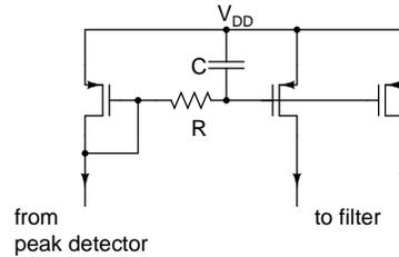
Figure 8.45: Filtering the dynamic bias current.
