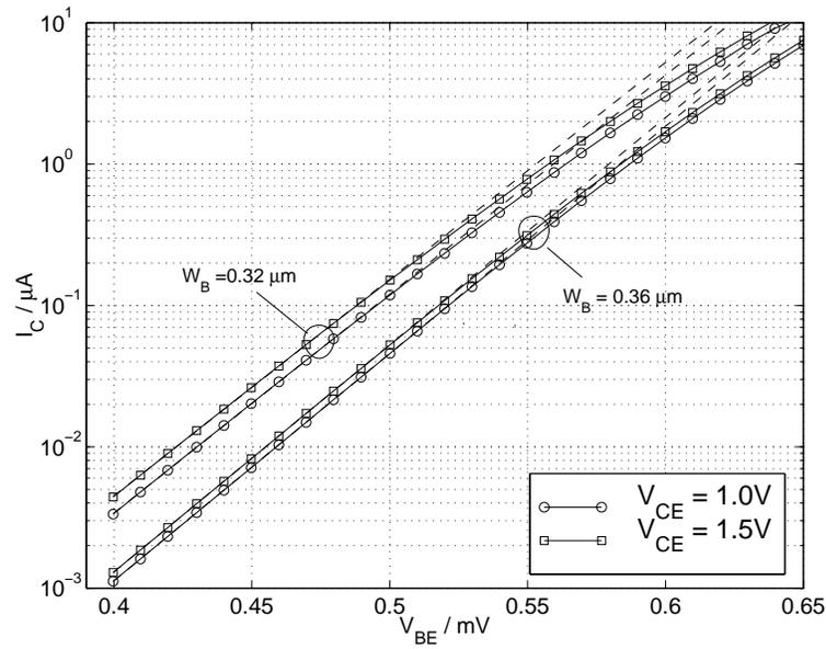
Figure 8.32: Characteristics of the lateral pnp transistor with its base and gate tied together.
