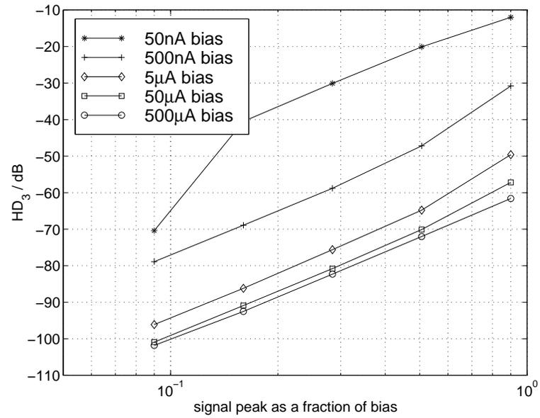
Figure 7.27: Third harmonic distortion as a function of the modulation index for various values of bias currents.
