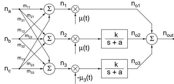
Figure 6.9: Model for calculating the output noise due to correlated noise sources.
