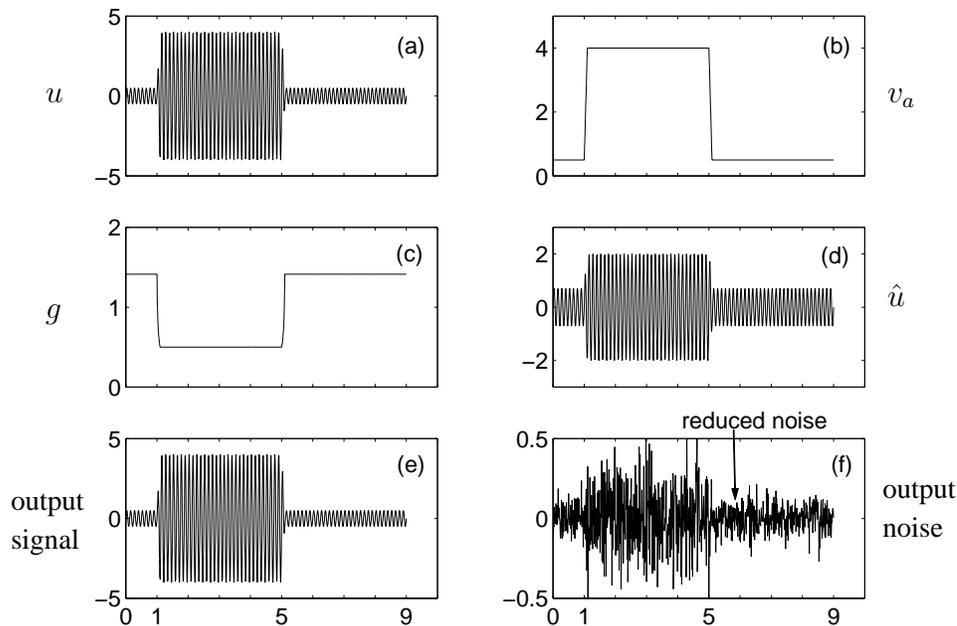
Figure 4.3: Syllabic companding under ideal conditions: (a) Input  $u$  with a changing envelope, (b)  $v_a$ , the detected envelope of  $u$ , (c) Gain  $g$  of the input amplifier, (d) Compressed signal  $\hat{u}$ , (e) Output signal of the system, (f) Output noise of the system.
