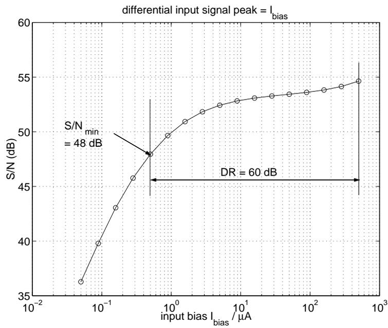
Figure 7.26: Signal to noise ratio with single ended signal peak at 50% of the bias
