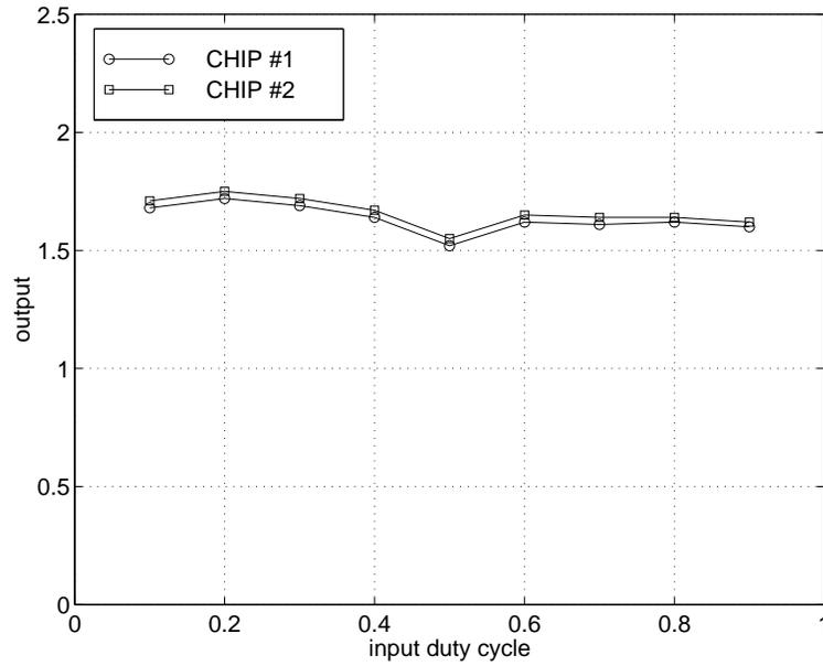
Figure 8.30: Outputs of two coupled peak detectors operating in differential mode.
