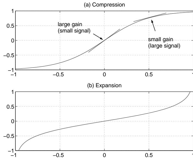
Figure 1.2: Comping using a nonlinearity: (a) Compression at the input, (b) Expansion at the output.
