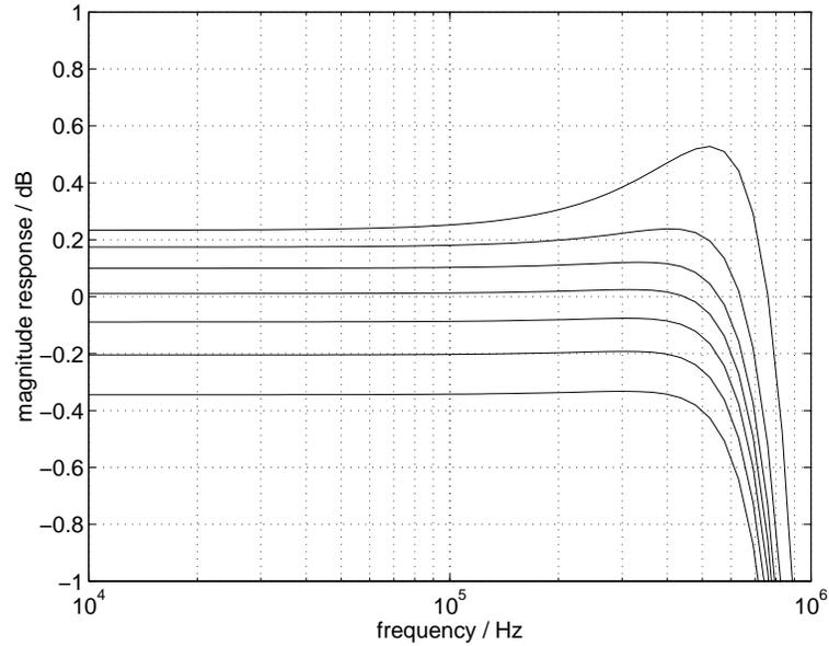
Figure 7.24: Passband detail of the frequency response with the bias current varied from 500 nA to 500  $\mu$ A.
