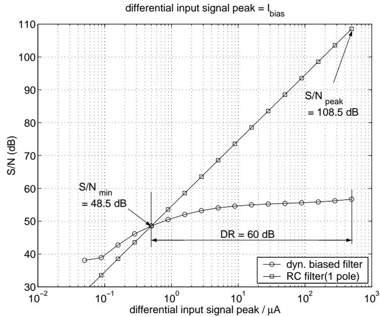
Figure 7.20: Signal to noise ratio of the log-domain and passive RC filters.
