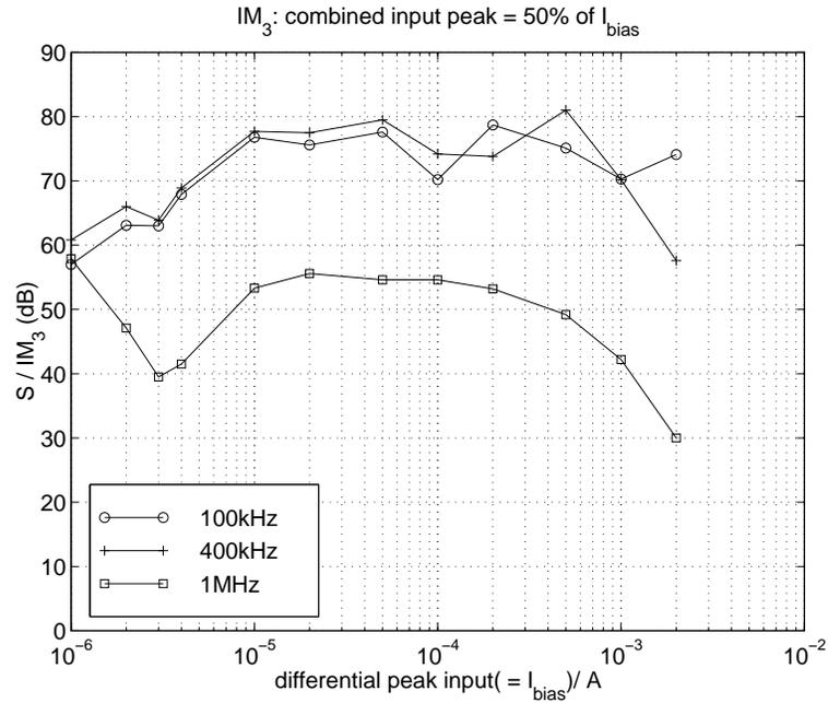
Figure 8.11: Measured third order intermodulation distortion versus input amplitude.
