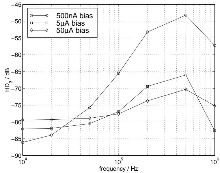
Figure 7.28: Third harmonic distortion as a function of frequency.
