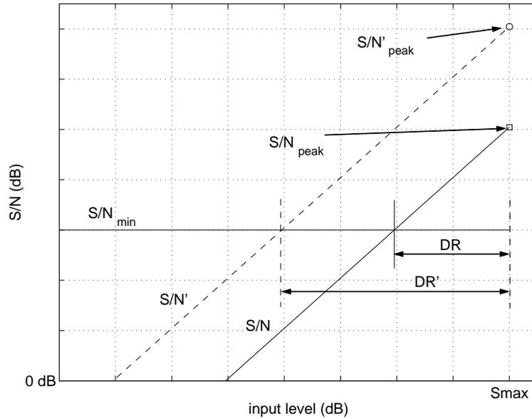
Figure 2.3: Signal to noise ratio and dynamic range of a typical active filter.
