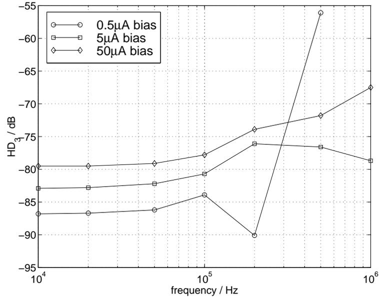
Figure 7.17: Third harmonic distortion as a function of frequency.
