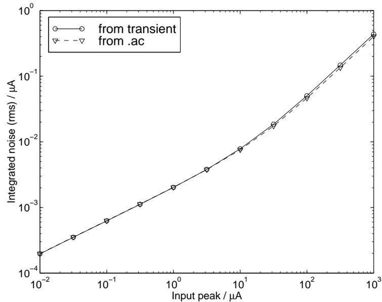
Figure 2.24: Integrated noise at the output of the filter in Fig. 2.21 with the input amplitude as a parameter: solid line—from transient analysis, dashed line—from “.AC” analysis.
