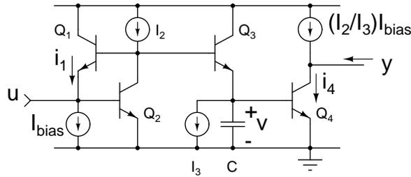
Figure 2.20: First-order filter in Fig. 2.7 with bias currents shown separately at the input and the output.
