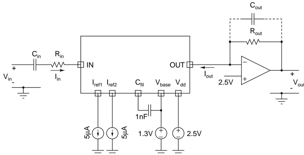
Figure 8.20: Measurement setup for the peak detector.
