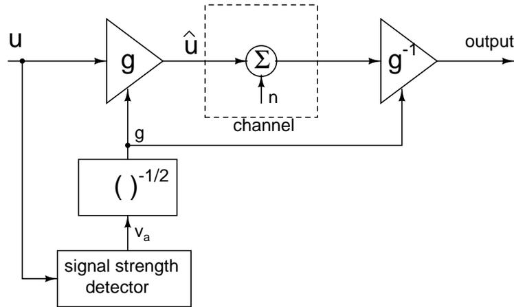
Figure 4.2: Companding with memoryless noisy channels.
