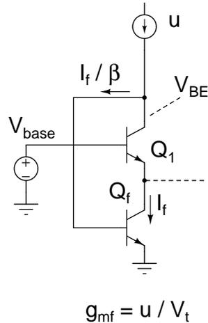
Figure 7.5: Feedback circuit used in [22] to establish the collector currents.
