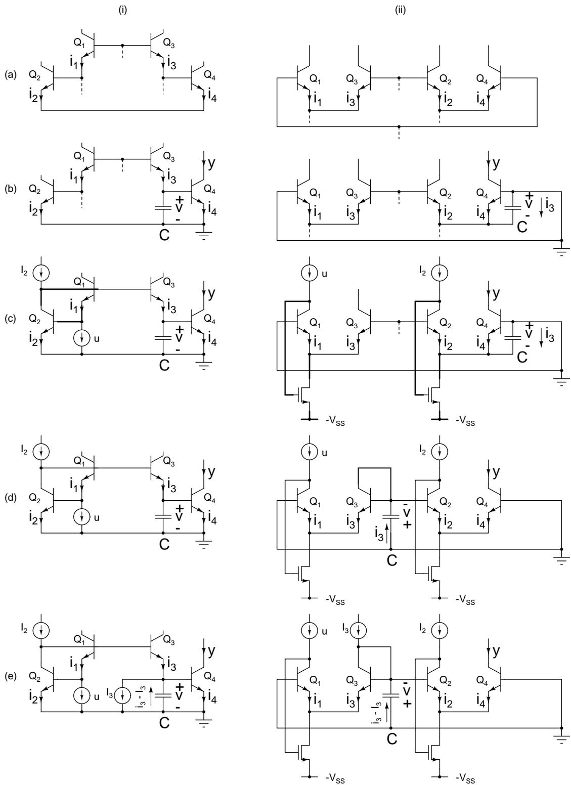
Figure 2.14: Deriving an alternative topology of a first-order log-domain filter.
