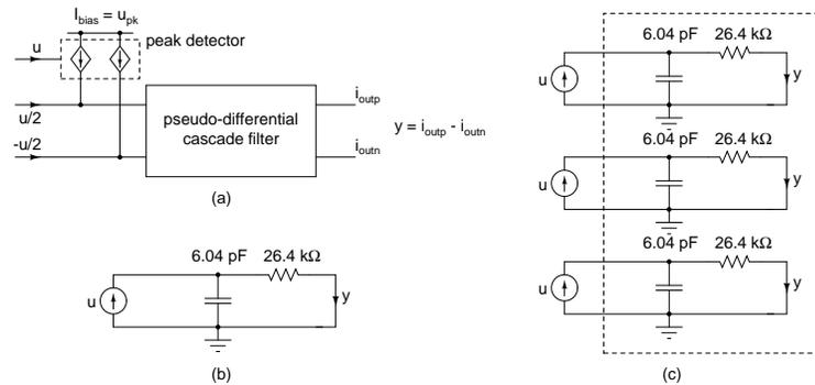
Figure 7.29: (a) Pseudo differential cascade filter biased from an ideal peak detector, (b) Current mode RC filter with  $S/N = 48 \text{ dB}$  for a  $0.5 \mu\text{A}$  peak input, (c) Three first-order RC filters.
