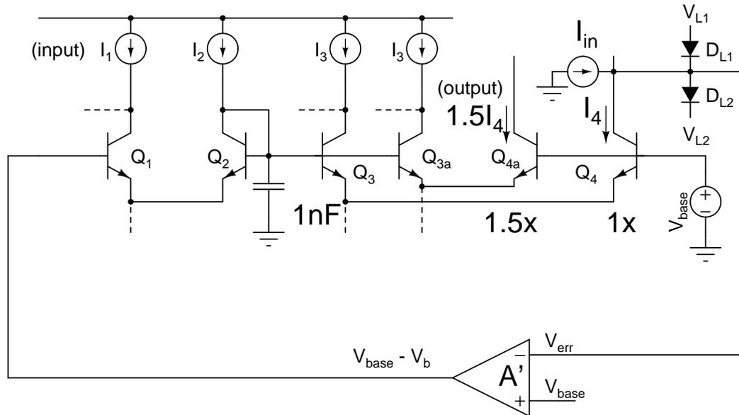
Figure 7.38: Complete circuit of the peak detector.
