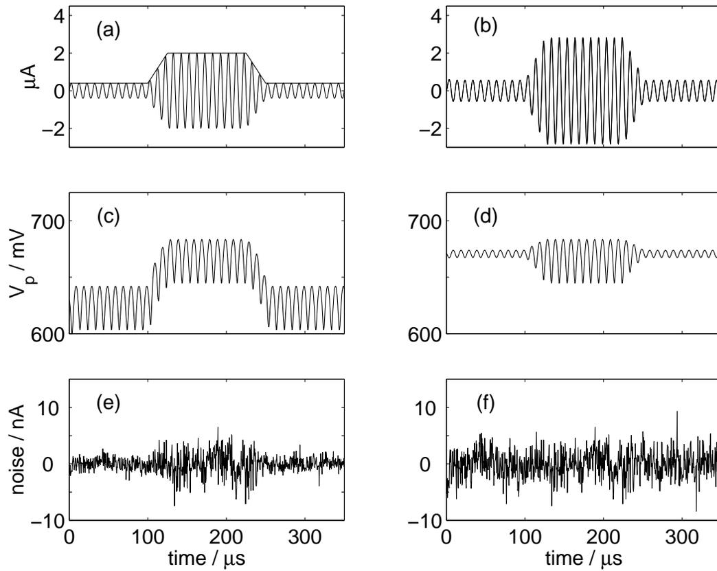
Figure 3.4: Results of simulation of the circuit in Fig. 3.1(b): (a) Input  $u$  and its envelope, (b) Differential output, (c)  $v_p$  with dynamic bias, (d)  $v_p$  with a constant bias, (e) Output noise with a dynamic bias, (f) Output noise with a constant bias.
