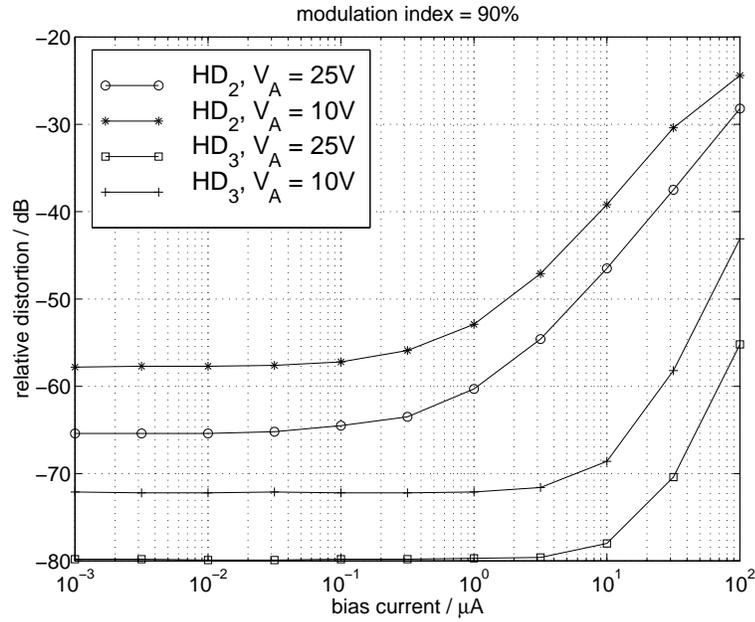
Figure 7.9: Distortion vs. bias for a constant modulation index and two Early voltages.
