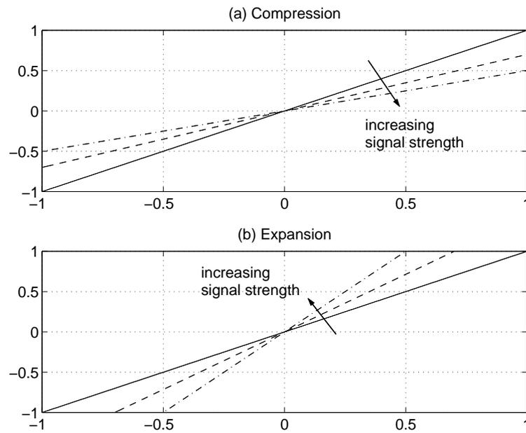
Figure 1.3: Comping using parameterized gains (a) Compression at the input, (b) Expansion at the output.
