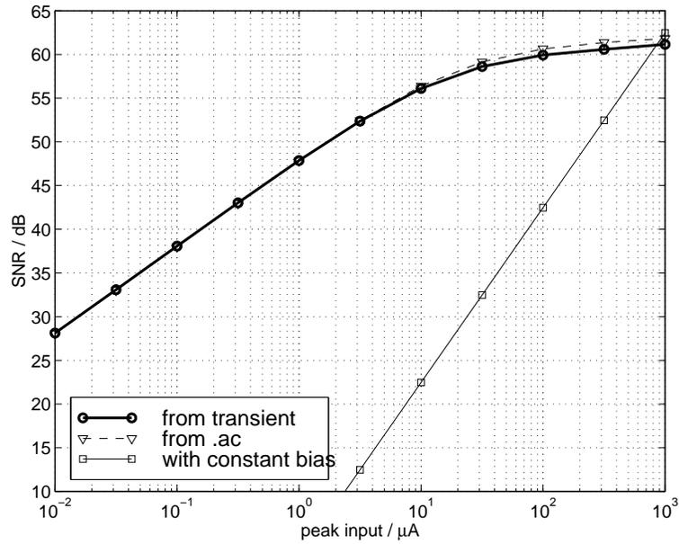
Figure 2.25: Signal to noise ratio at the output of the filter in Fig. 2.21.
