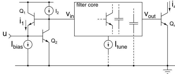
Figure 3.3: Generic structure of a high order log-domain filter
