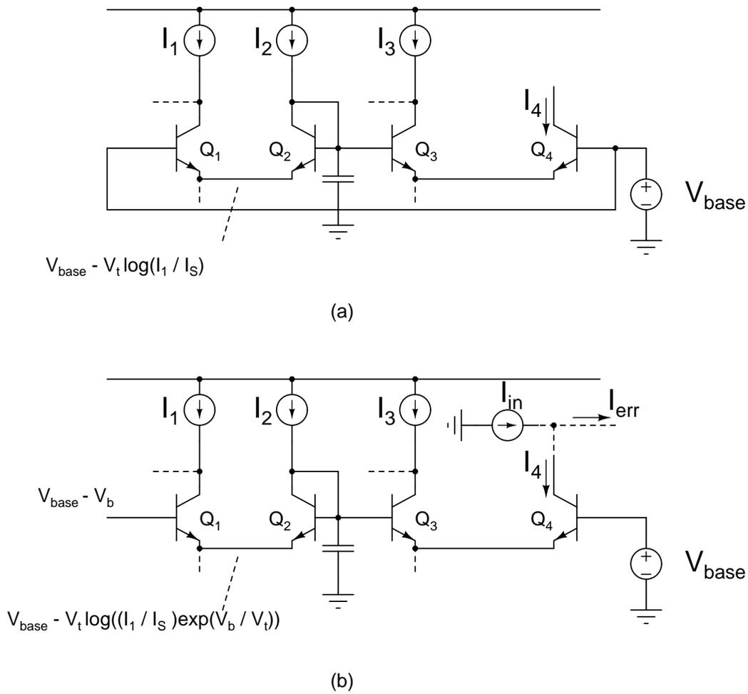
Figure 7.35: Combination of an exponentiator and a low pass filter.
