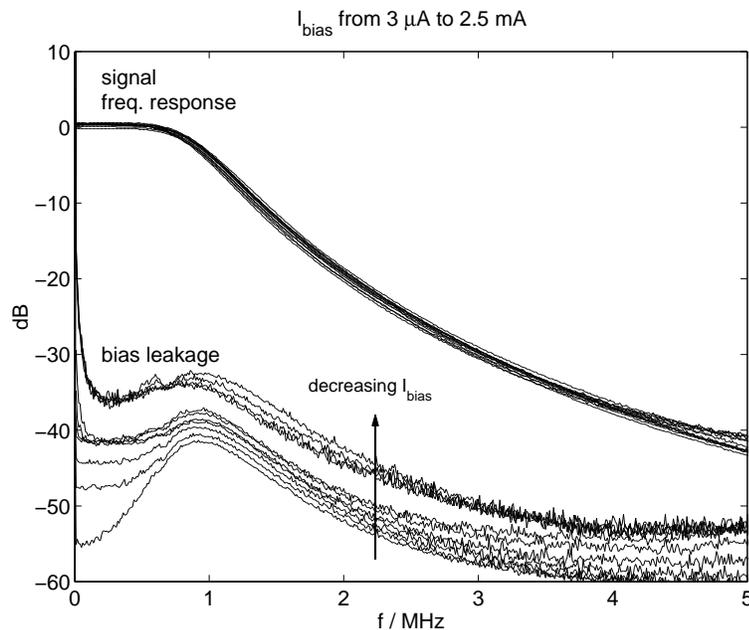
Figure 8.3: Response at the differential output of the filter to common mode and differential inputs.
