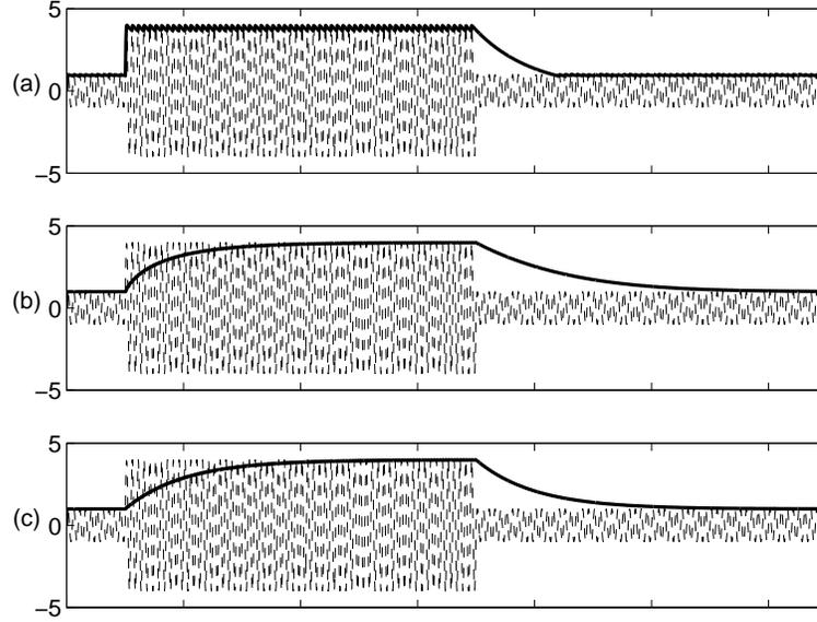
Figure 4.9: Responses of (a) Classical diode-RC peak detector, (b) RMS detector, (c) Rectifier and averaging, to a sinusoidal input with a changing amplitude. The time constant used in the filters in Fig. 4.7(a-i), Fig. 4.7(b-i) and Fig. 4.7(c) is ten times as long as the period of the input.
