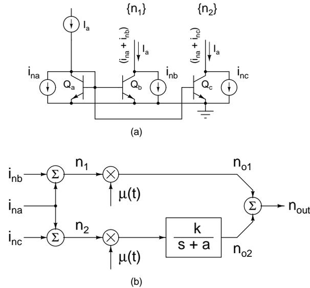
Figure 6.8: (a) Current mirror with correlated output noise, (b) Equivalent circuit.
