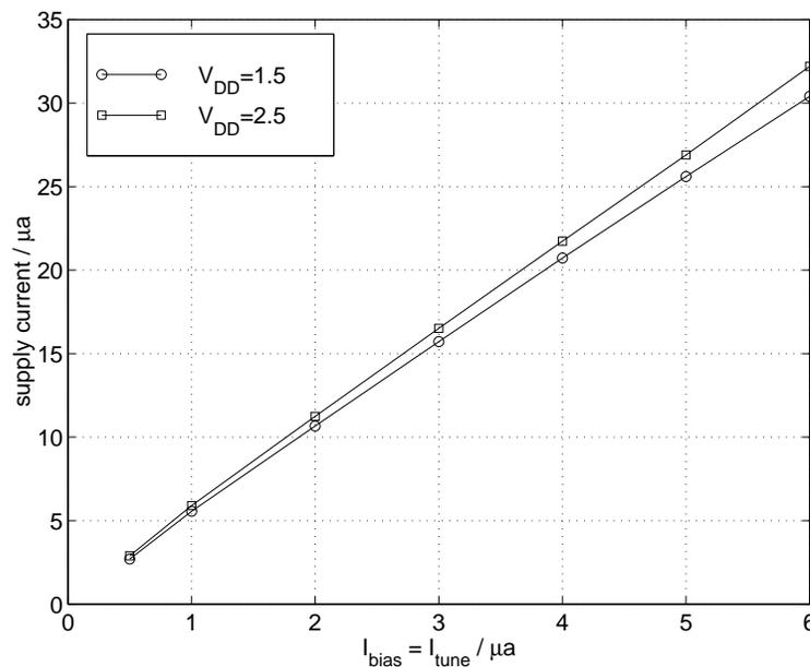
Figure 8.39: Current consumption of the second-order filter.
