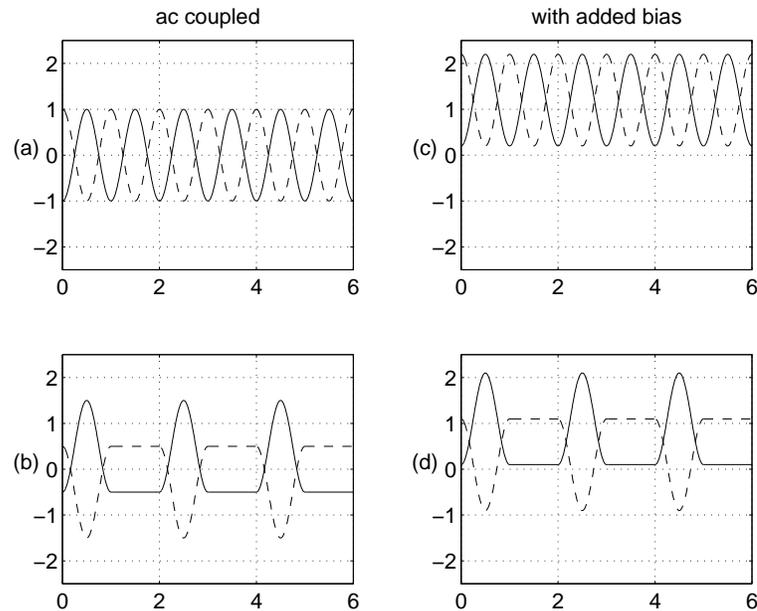
Figure 7.42: (a) Differential signal with equal positive and negative peaks, (b) Differential signal with unequal positive and negative peaks, (c) (a) with added bias, (d) (b) with added bias.
