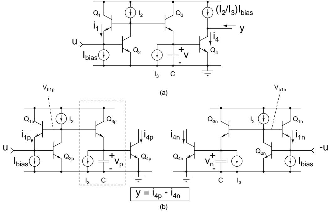
Figure 3.1: (a) First order log-domain filter, (b) Pseudo-differential operation with time varying bias.
