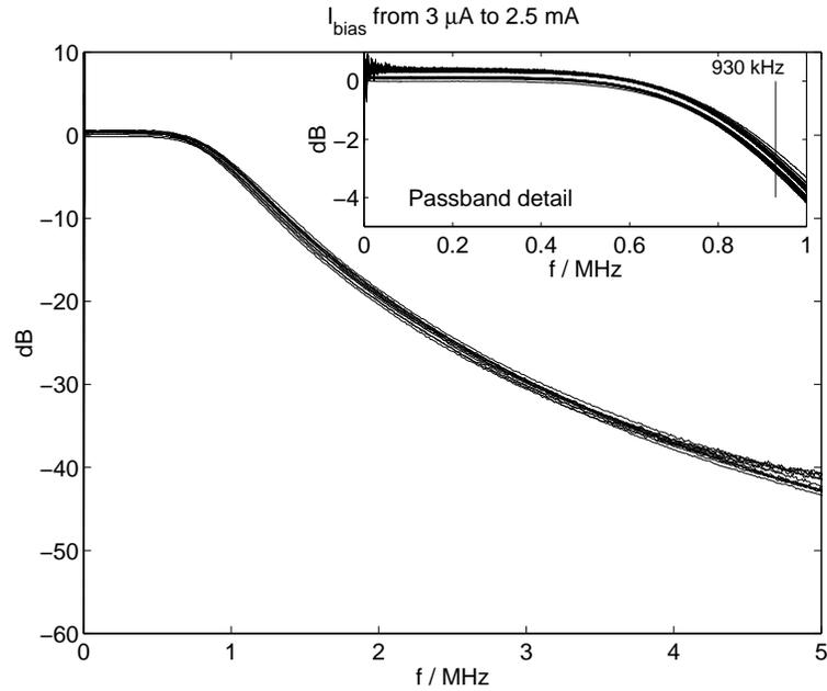
Figure 8.2: Frequency response of the fabricated third order pseudo-differential Butterworth ladder filter.
