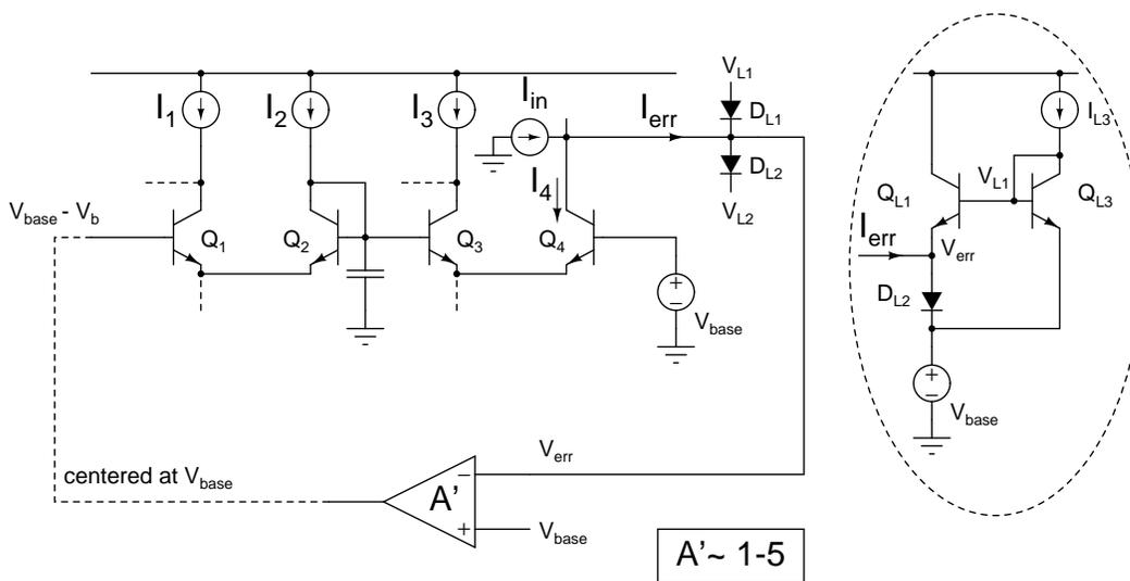
Figure 7.36: Negative feedback around the exponentiator and the low pass filter.
