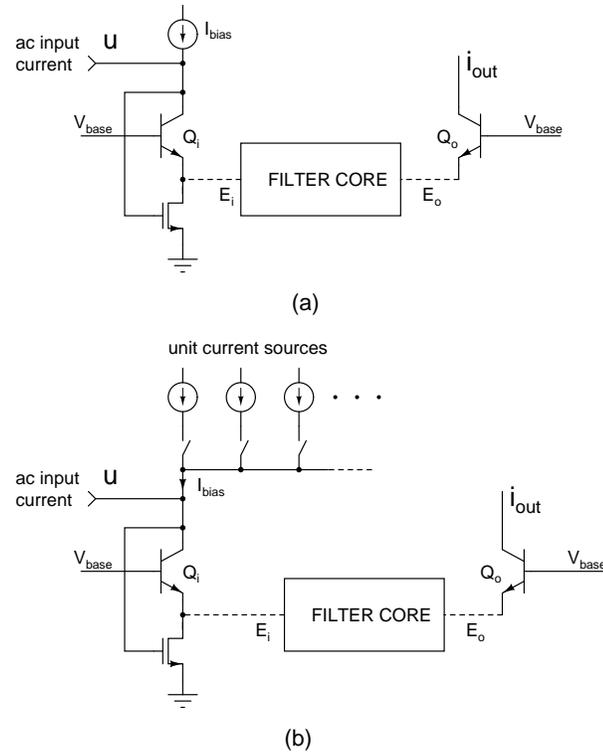
Figure 8.42: (a) Log-domain filter drawn in a general form, (b) Dynamic biasing in discrete steps.
