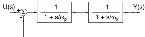
Figure 7.46: Block diagram of a second-order Butterworth filter using two lossy integrators.
