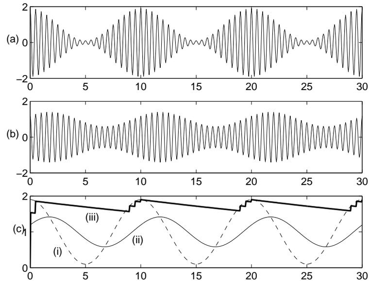
Figure 4.11: (a) Amplitude modulated signal, (b) Output when (a) is passed through a bandpass filter with  $Q = 10$ , (c-i) Envelope of (a), (c-ii) Envelope of (b), (c-iii) Envelope of (a) as detected by a “slow” peak detector.
