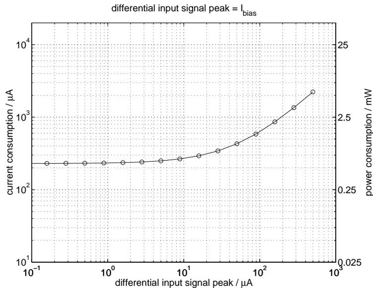
Figure 7.19: Power consumption of the pseudo-differential log-domain filter.
