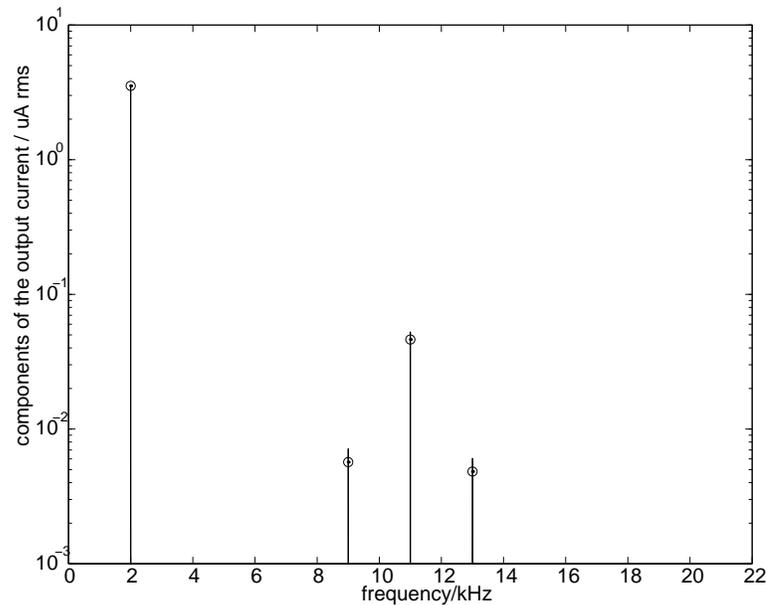
Figure 6.12: Intermodulation due to sinusoidal interference—lines: calculated, circles: measured.
