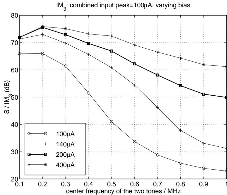
Figure 8.10: Measured third order intermodulation distortion versus frequency with a single ended input peak of  $100 \mu\text{A}$  and values of bias current  $I_{bias}$  shown in the insert.
