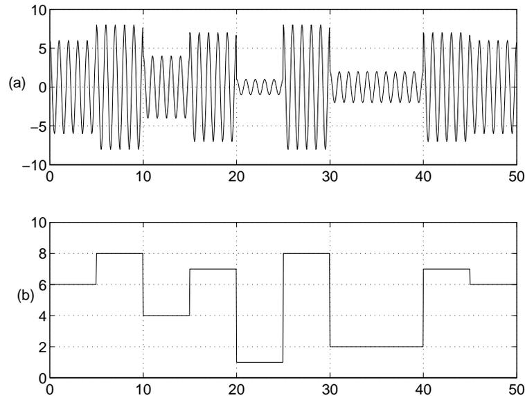
Figure 4.1: (a) Amplitude shift keyed waveform, (b) Envelope of (a).
