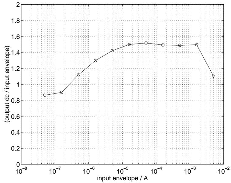
Figure 7.40: Simulated ratio of the dc output to the input peak.
