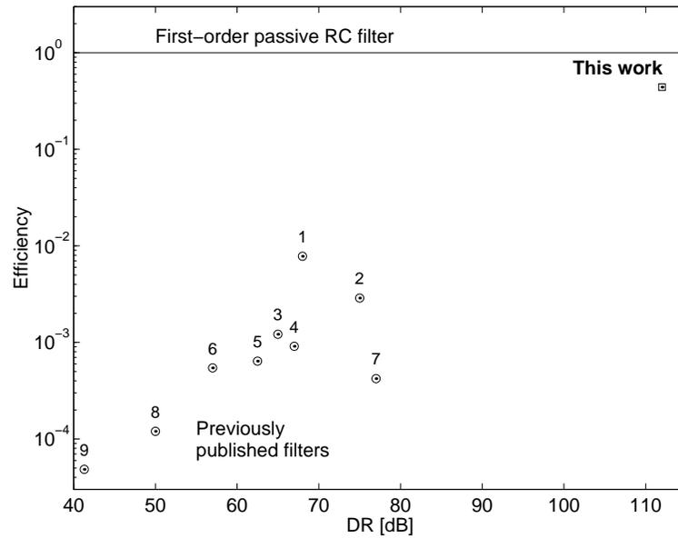
Figure 8.18: Efficiency when compared to a first-order passive RC filter.
