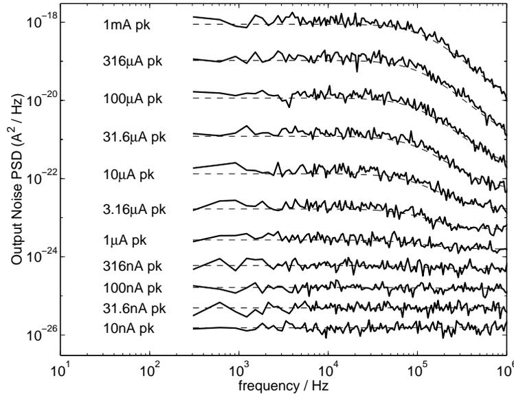
Figure 2.23: Noise PSD at the output of the filter in Fig. 2.21: solid line—from transient analysis, dashed line—from “.AC” analysis.
