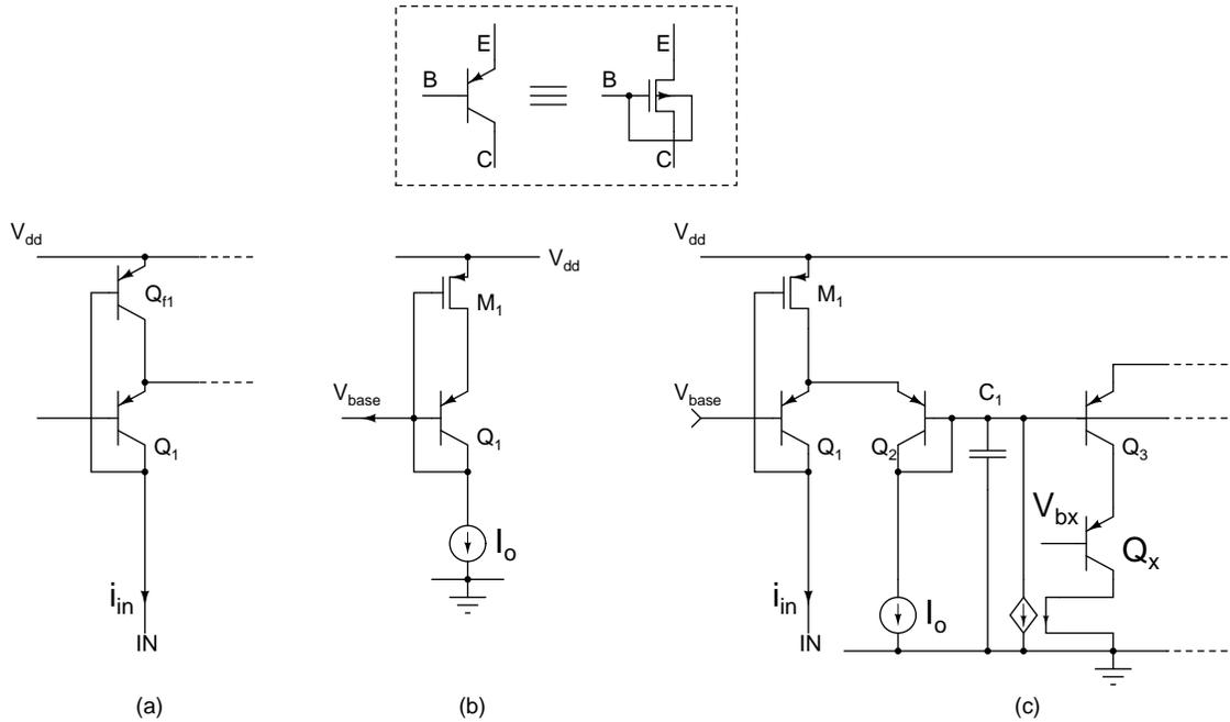
Figure 8.46: (a) Using a lateral PNP transistor instead of a pMOS transistor to increase the  $g_m$  of the feedback path, (b) Generating  $V_{base}$ , (c) Using a cascode transistor equalize collector voltages of all the transistors.
