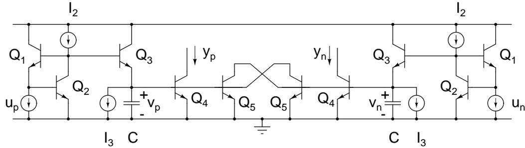
Figure 2.12: Class-AB instantaneous companding log-domain filter.
