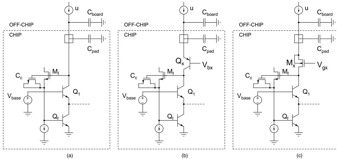
Figure 8.44: (a) Existing input stage with pad and board parasitics, (b) Using a PNP transistor at the input to isolate the board parasitics, (c) Using a pMOS transistor at the input to isolate the board parasitics.
