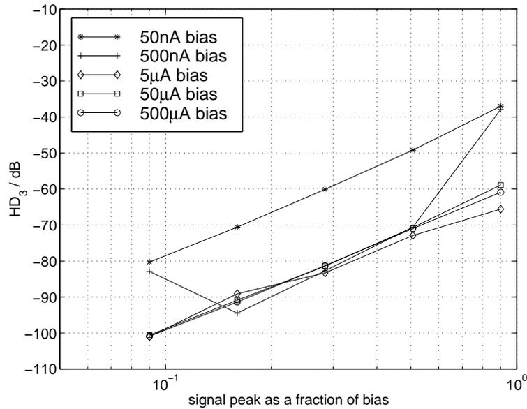
Figure 7.16: Third harmonic distortion as a function of bias.
