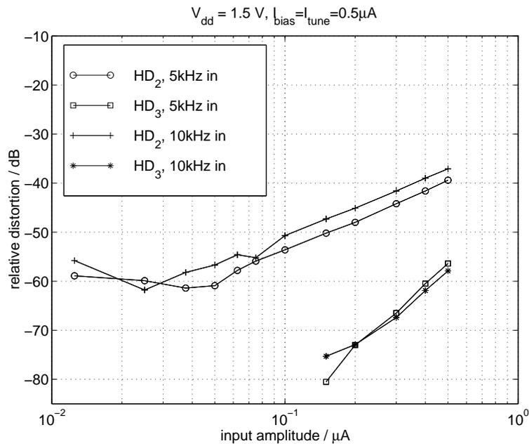
Figure 8.35: Distortion performance of the filter with 0.5  $\mu\text{A}$  bias current.
