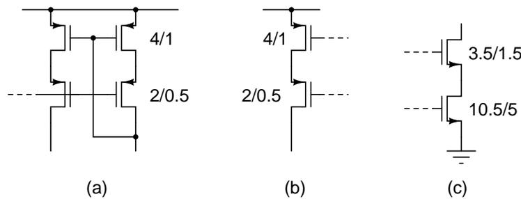
Figure 7.10: (a) Current mirror, (b) Current source, (c) Current sink.
