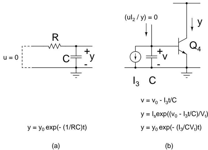
Figure 2.9: Damping in a log-domain filter.
