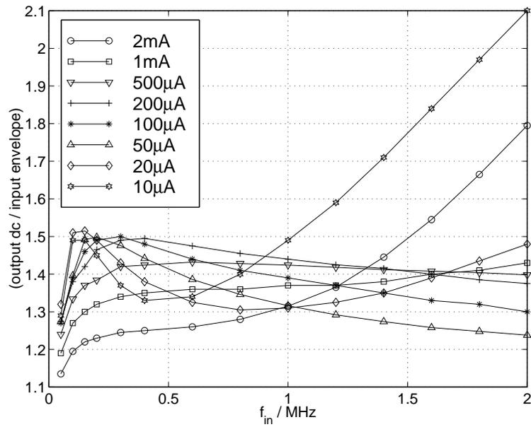
Figure 8.23: Frequency response of the peak detector.
