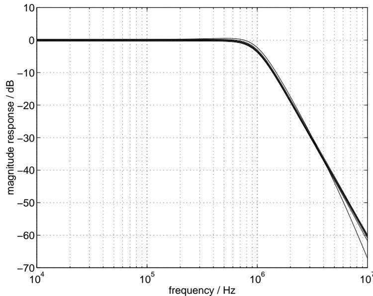
Figure 7.23: Frequency response with the bias current varied from 500 nA to 500  $\mu$ A.
