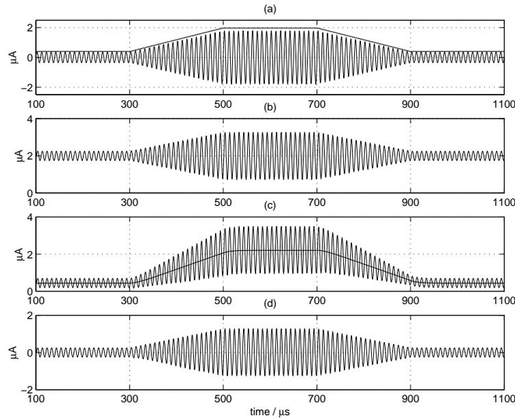
Figure 2.22: Simulation of the filter in Fig. 2.21: (a) Input  $u$  with a changing envelope and the corresponding  $u_R$ , (b) Output transistor current in the filter with a constant bias, (c) Output transistor current and the output bias current  $mI_{bias}$  in the filter with a dynamic bias, (d) Output signal  $y$  of the filter for cases (b) and (c).
