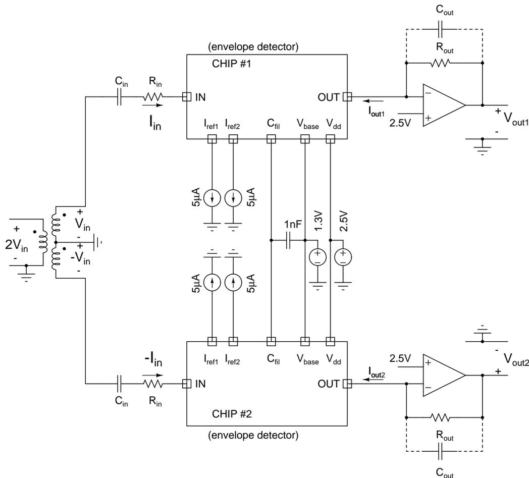
Figure 8.28: Setup to measure a differentially responding peak detector.
