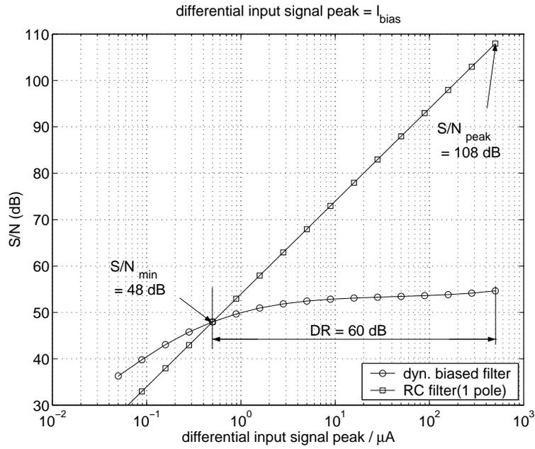
Figure 7.31: Signal to noise ratio of the log-domain and passive RC filters.
