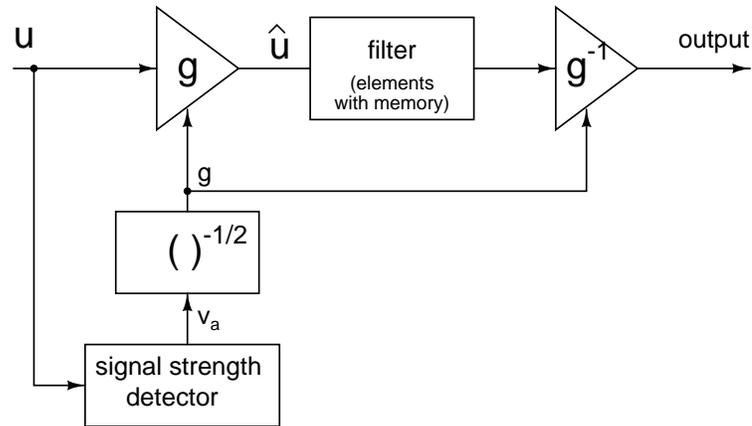
Figure 4.5: Companding filter with memory elements between the compressor and the expander.
