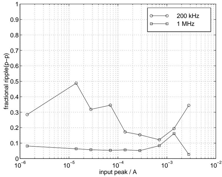
Figure 8.22: Peak-peak ripple at the output with 200 kHz and 1 MHz inputs.
