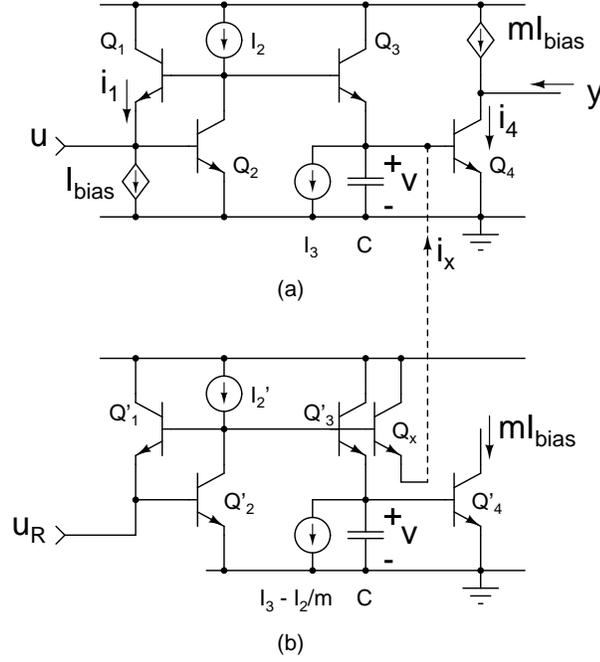
Figure 2.21: (a) First order log-domain filter with a current  $i_x$  injected into the capacitor, (b) Circuit for generating  $i_x$  and the filter used to average  $I_R$ .
