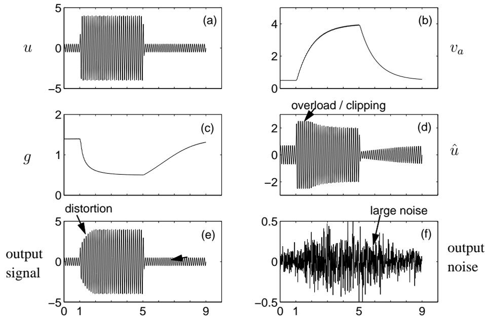
Figure 4.4: Syllabic companding under practical conditions: (a) Input  $u$  with a changing envelope, (b)  $v_a$ , the detected envelope of  $u$ , (c) Gain  $g$  of the input amplifier, (d) Compressed signal  $\hat{u}$ , (e) Output signal of the system, (f) Output noise of the system.
