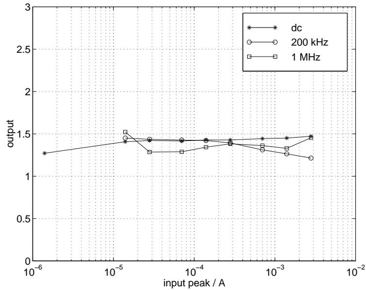
Figure 8.21: Output dc component with dc, 200 kHz and 1 MHz inputs.
