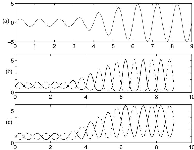
Figure 3.6: (a) Input with a changing envelope, (b) Geometrically split inputs for a class-AB filter, (c) Input with a dynamic bias added to it.
