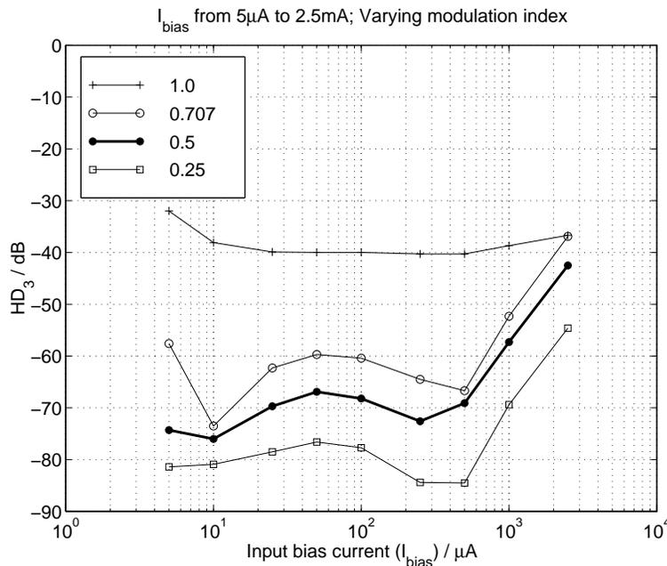
Figure 8.8: Measured third harmonic relative to the fundamental with a 400 kHz input for modulation index values shown in the insert.
