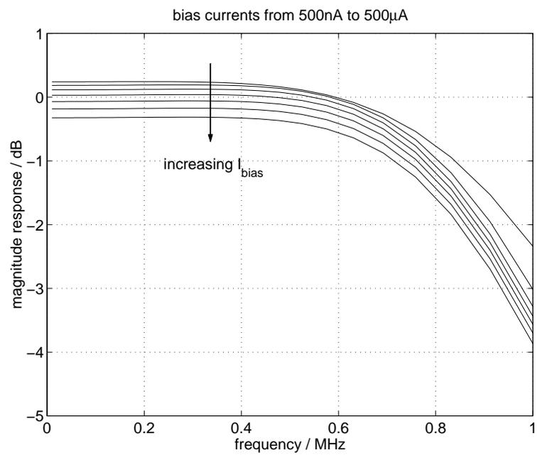
Figure 7.13: Passband detail of the frequency response with the bias current varied from 500 nA to 500  $\mu$ A.
