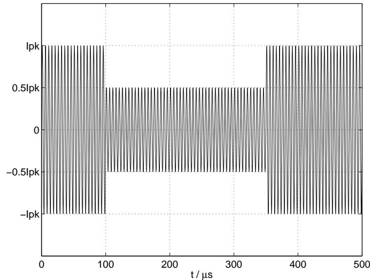
Figure 8.24: Input used to measure the attack and the decay times of the peak detector.
