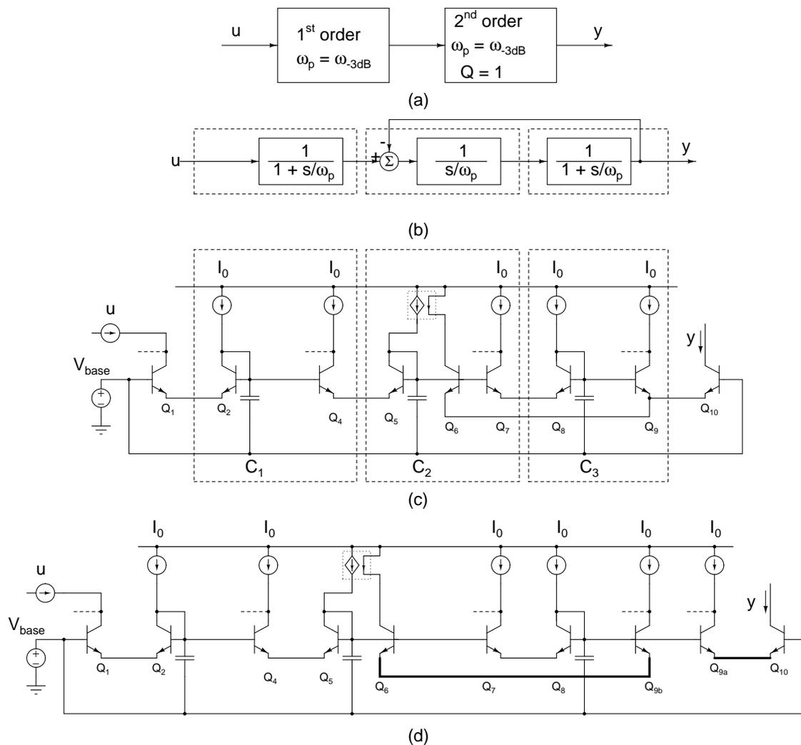
Figure 7.22: Third-order Butterworth filter: (a) Cascade prototype, (b) Block diagram using first order stages, (c) Log-domain realization, (d) Separating the feedback and feed-forward paths.
