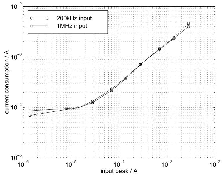
Figure 8.26: Current consumption of the peak detector.
