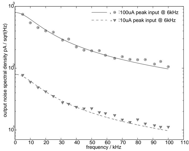
Figure 6.14: Output noise of a first order class-B filter—lines: calculated, circles: measured.
