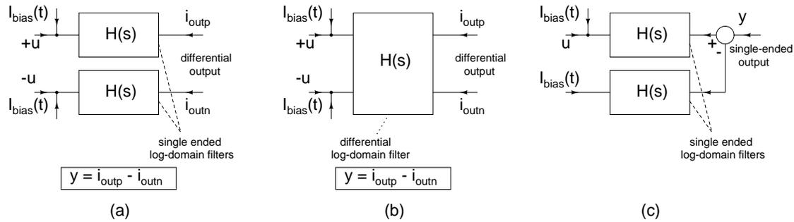
Figure 3.2: Distortionless dynamic biasing: (a) Pseudo-differential operation, (b) Using differential (class-AB) filters, (c) Single ended operation.
