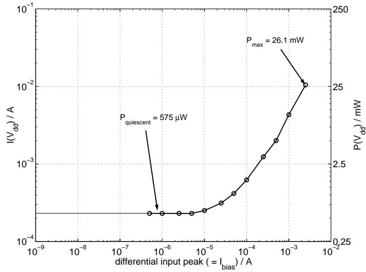
Figure 8.13: Measured current and power consumption of the filter.
