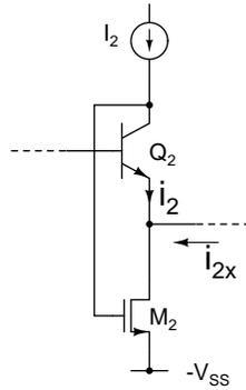
Figure 2.15: Feedback around  $Q_2$  in Fig. 2.14 to force a current into its collector.
