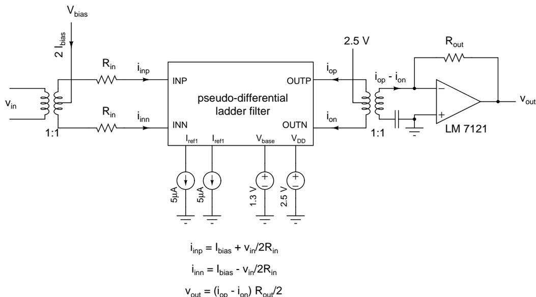
Figure 8.1: Setup used to measure the pseudo-differential ladder filter.
