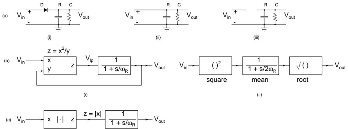
Figure 4.7: Techniques for envelope detection: (a) Classical diode-RC peak detector, (b) RMS detector, (c) Rectifier and averaging.
