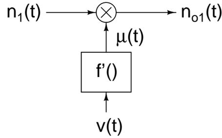
Figure 6.3: Noise equivalent circuit for Fig. 6.2(a).
