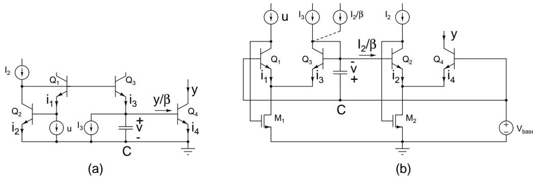
Figure 7.1: First order log-domain filter topologies (a) From [6], (b) From [19].
