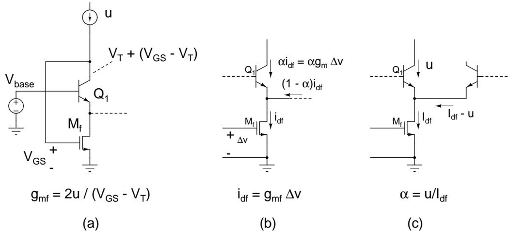
Figure 7.4: Feedback to establish the collector currents (a) From [19], (b, c) Small signal picture of (a).
