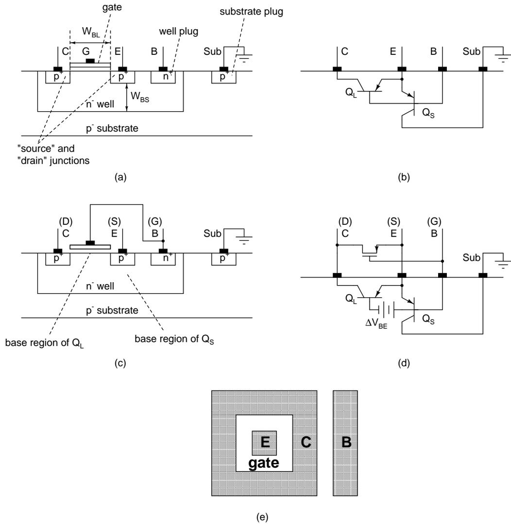
Figure 5.1: (a) Simplified cross section of a conventional lateral PNP transistor, (b) Electrical equivalent of (a), (c) Simplified cross section of an enhanced lateral PNP transistor, (d) Electrical equivalent of (c), (e) Top view of a practical lateral transistor.
