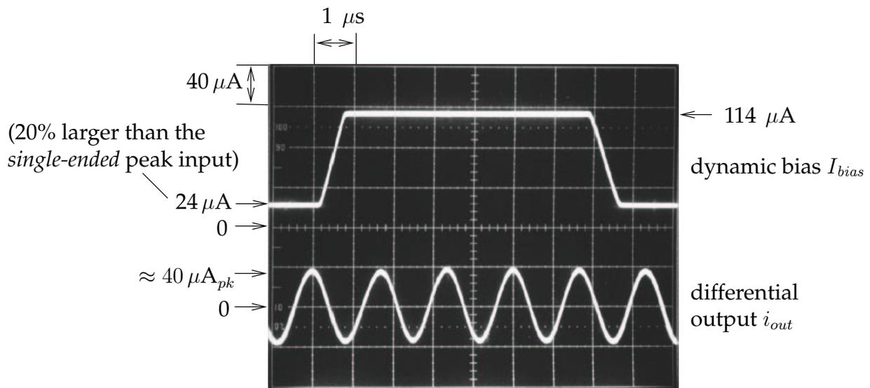
Figure 8.12: Time varying bias current and the resulting differential output of the pseudo-differential filter.
