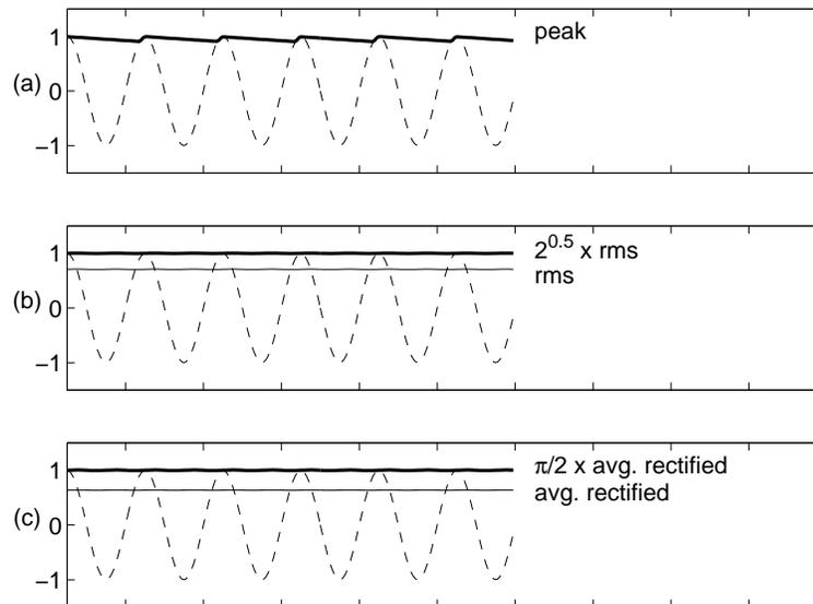
Figure 4.8: Steady state responses of (a) Classical diode-RC peak detector, (b) RMS detector, (c) Rectifier and averaging, to a sinusoidal input. The time constant used in the filters in Fig. 4.7(a-i), Fig. 4.7(b-i) and Fig. 4.7(c) is ten times as long as the period of the input.
