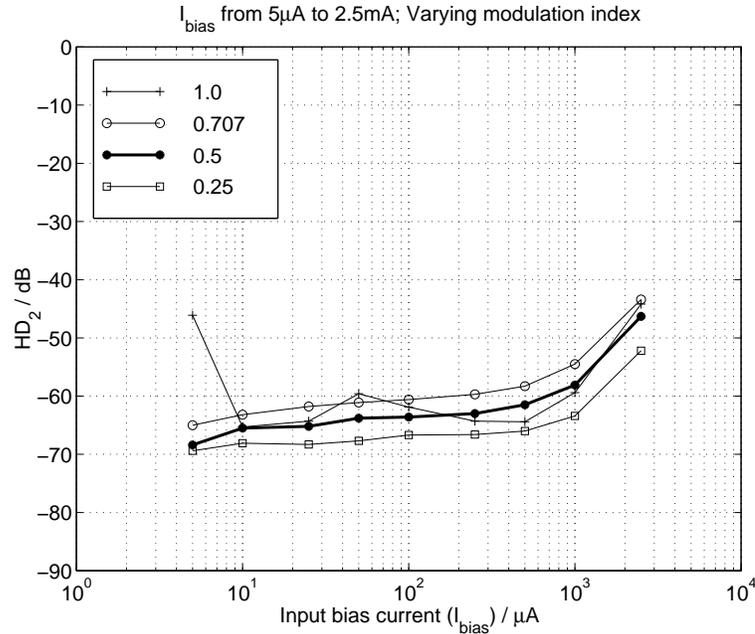
Figure 8.7: Measured second harmonic relative to the fundamental with a 400 kHz input for modulation index values shown in the insert.
