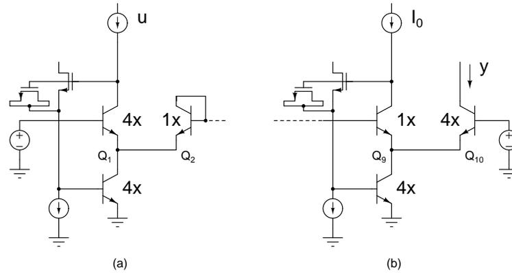
Figure 7.7: Transistor sizing at the (a) input, (b) output.
