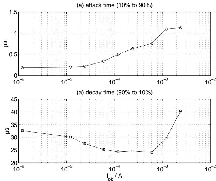
Figure 8.25: (a) Attack time and (b) Decay time of the peak detector as a function of the bias current.
