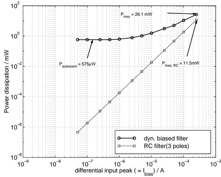
Figure 8.16: Power dissipation versus the input signal: Pseudo-differential ladder filter and passive RC filter.
