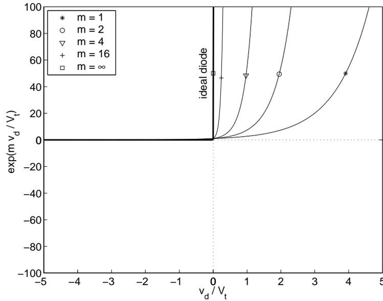
Figure 7.34: Diode characteristics
