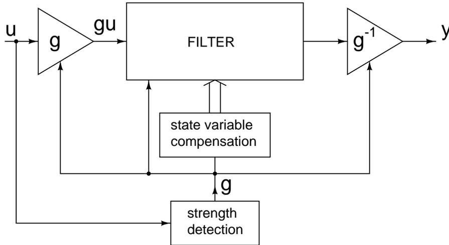
Figure 2.19: Block diagram of a general syllabic companding filter.
