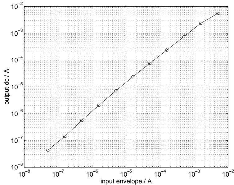
Figure 7.39: Simulated dc output of the peak detector vs. input peak.
