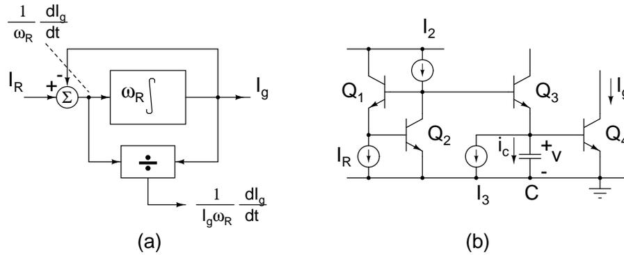
Figure 2.18: Generating the time derivative of the gain control current  $I_g$ .
