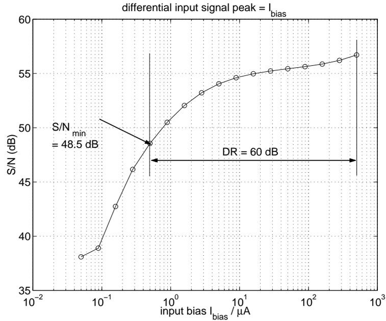
Figure 7.15: Signal to noise ratio with single ended signal peak at 50% of the bias.
