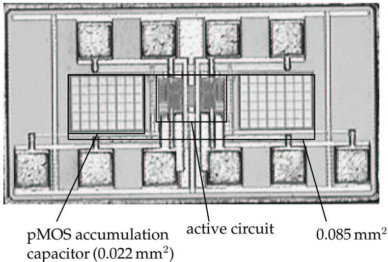
Figure 8.40: Photograph of the 2<sup>nd</sup> order filter chip using lateral PNP transistors and pMOS accumulation capacitors.
