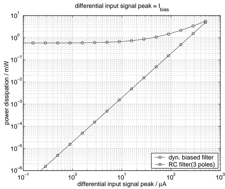
Figure 7.32: Power dissipation versus the input signal: Pseudo-differential cascade filter (Fig. 7.29(a)) and passive RC filter (Fig. 7.29(c)).
