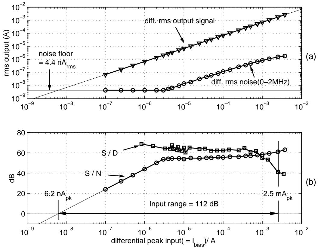
Figure 8.9: Measured noise (in 0-2 MHz band), SNR and THD.
