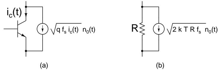
Figure 6.17: (a) Noise model of a transistor, (b) Noise model of a resistor.
