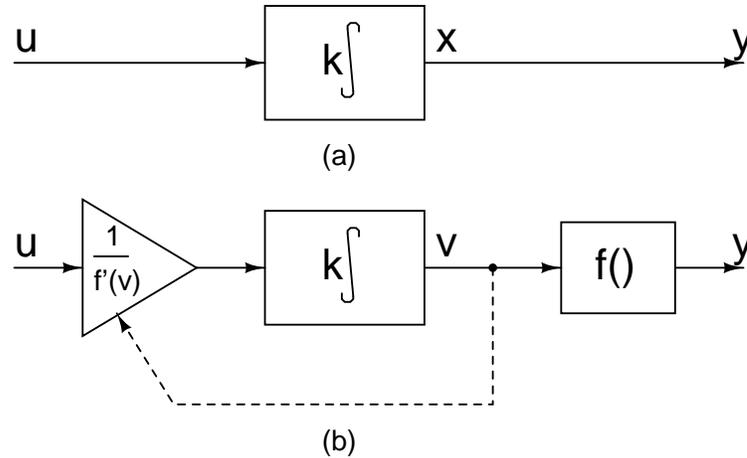
Figure 2.5: (a) Internally linear integrator, (b) ELIN integrator.
