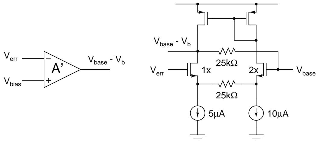
Figure 7.37: Inverting amplifier used in the feedback path of the peak detector.
