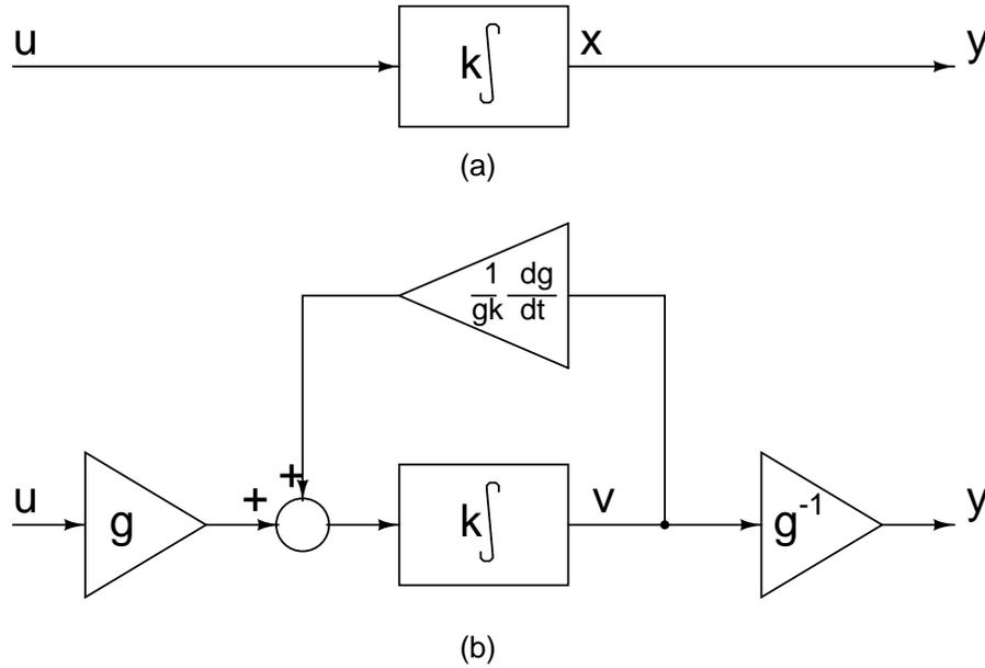
Figure 2.17: (a) Integrator, (b) Integrator with time varying gains at the input and the output.
