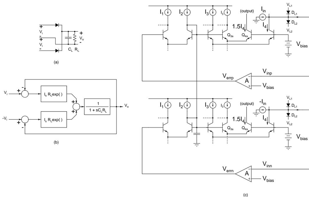
Figure 7.43: Peak detector with differential inputs.
