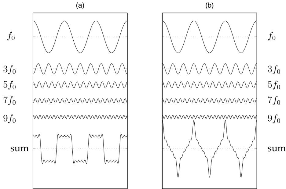
Figure 4.6: (a) First five harmonics of a square wave and their sum, (b) Same as (a), but with the third and seventh harmonic inverted.
