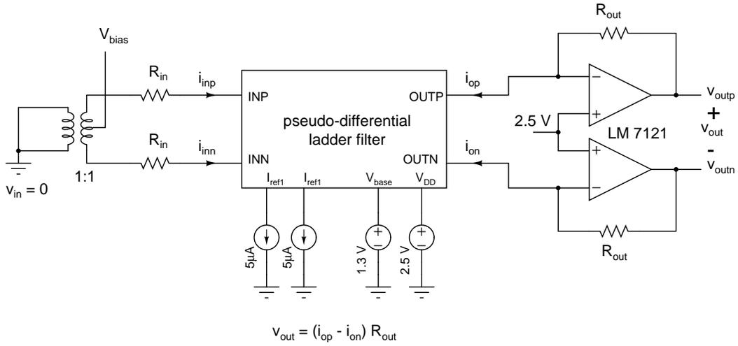
Figure 8.5: Measurement setup used to measure the output noise of the filter.
