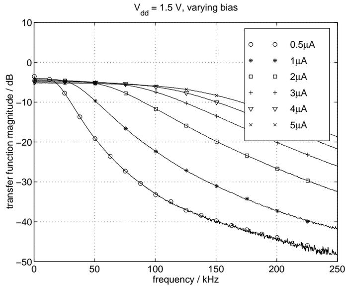
Figure 8.34: Frequency response of the second-order filter with a supply voltage of 1.5 V for various values of  $I_{tune}$  ( $= I_{bias}$ ) shown in the insert.
