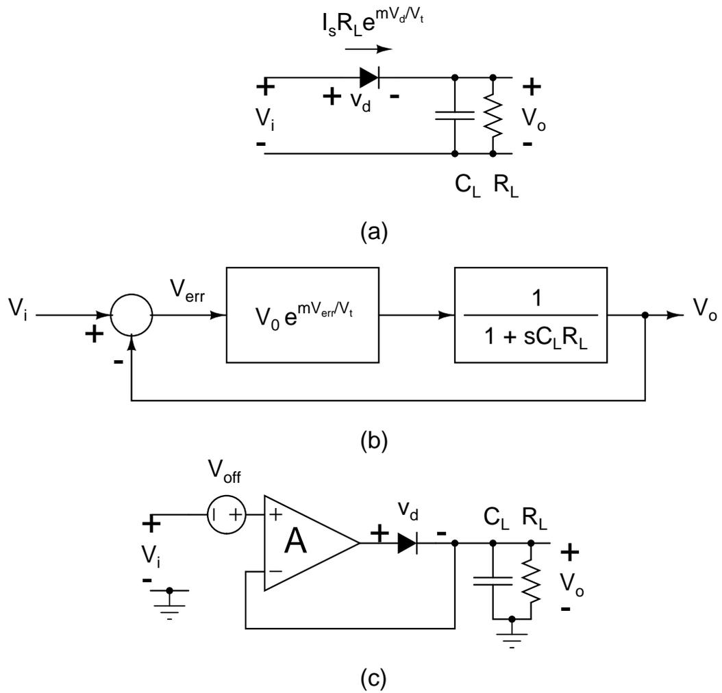
Figure 7.33: Principle of peak detection.
