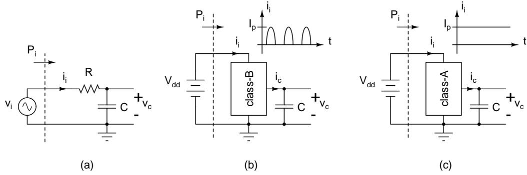
Figure A.1: (a) First-order RC filter, (b) Class-AB circuit driving a capacitor, (c) Class-A circuit driving a capacitor.
