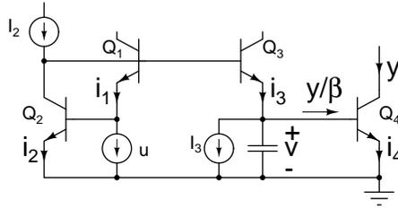
Figure 2.13: First order log-domain filter in Fig. 2.7(c).
