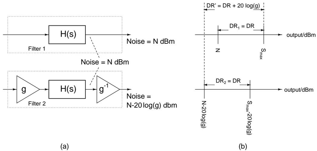
Figure 2.4: Filters with skewed operating ranges.
