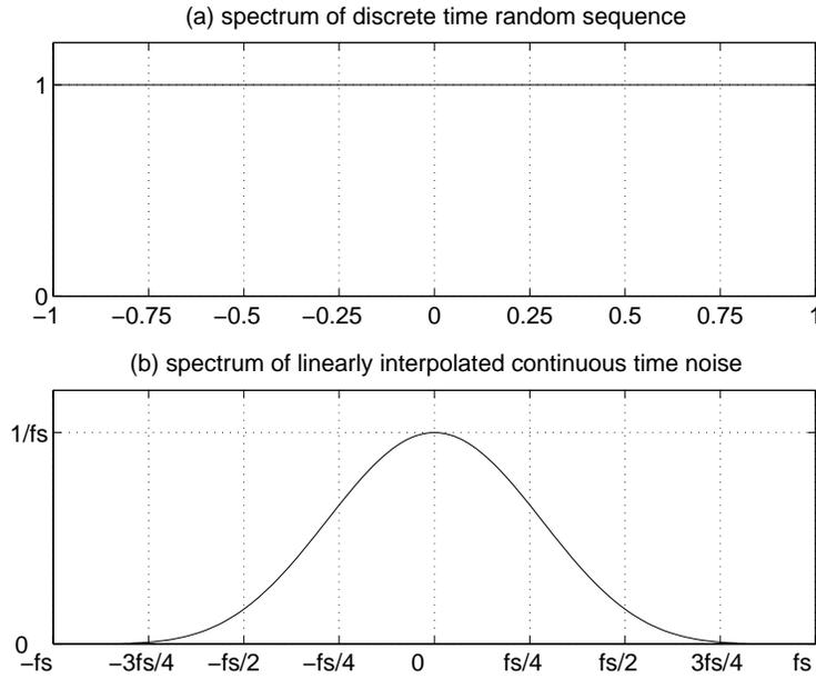
Figure 6.16: (a) Spectral density of discrete time uncorrelated sequence, (b) Spectral density of linearly interpolated continuous time waveform.
