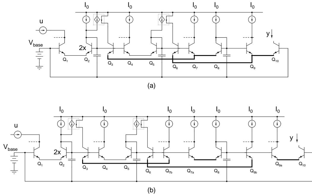
Figure 7.8: Separating the feedback and the feed-forward paths.
