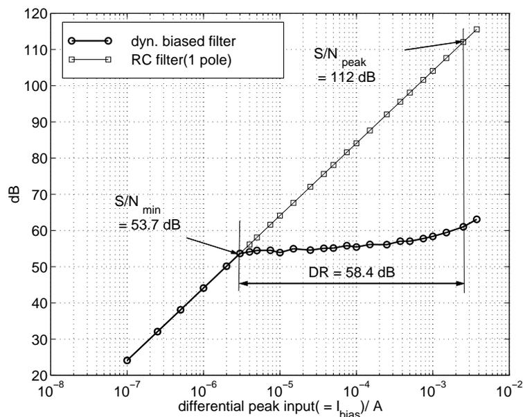
Figure 8.15: Signal to noise ratios of the pseudo-differential filter and the RC filter in Fig. 8.14.
