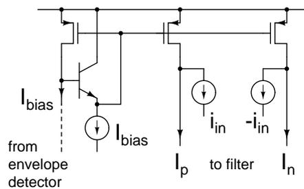
Figure 7.45: Biasing the filter from the peak detector.
