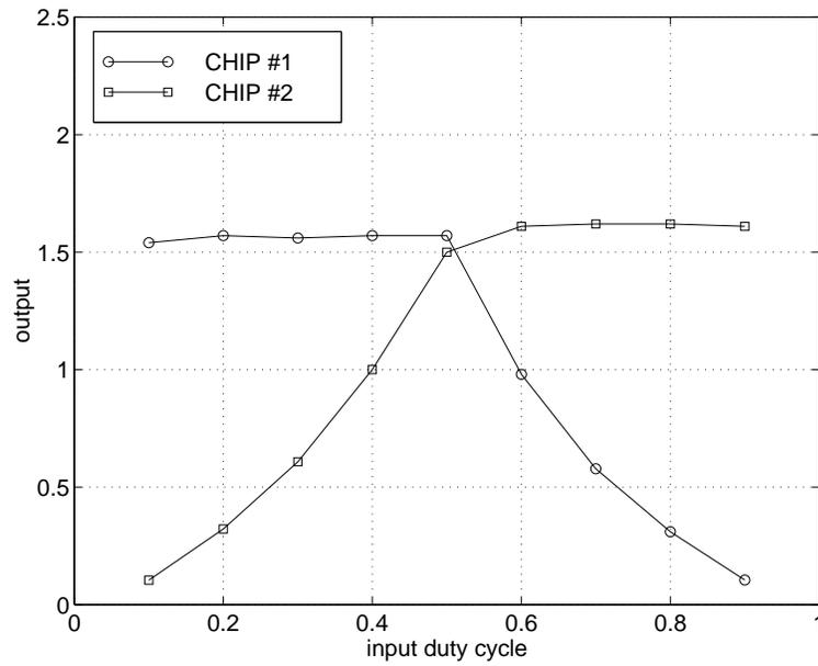
Figure 8.31: Outputs of the two peak detectors when they are uncoupled.
