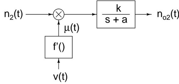
Figure 6.5: Noise equivalent circuit for Fig. 6.2(b).
