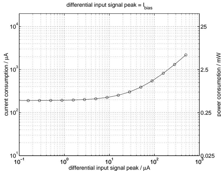
Figure 7.30: Power consumption of the pseudo-differential log-domain filter.
