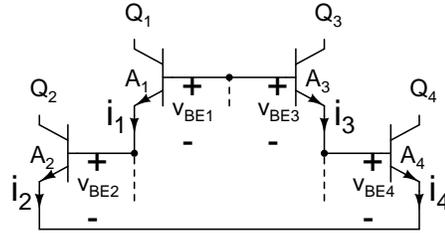
Figure 2.8: Translinear loop with four transistors.
