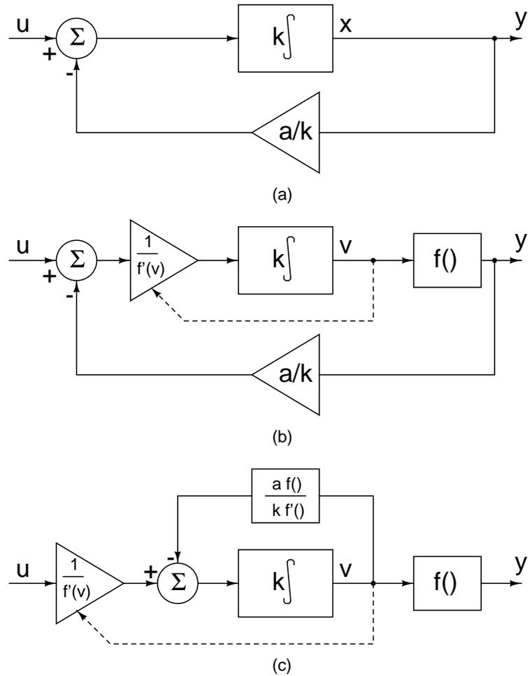
Figure 2.6: (a) Internally linear first-order filter, (b) ELIN first-order filter, (c) ELIN first-order filter with transformed feedback path.
