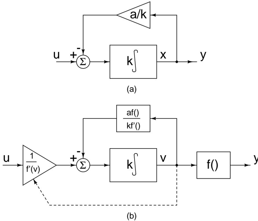
Figure 6.1: (a) Linear first order filter, (b) Instantaneous companding first order filter.
