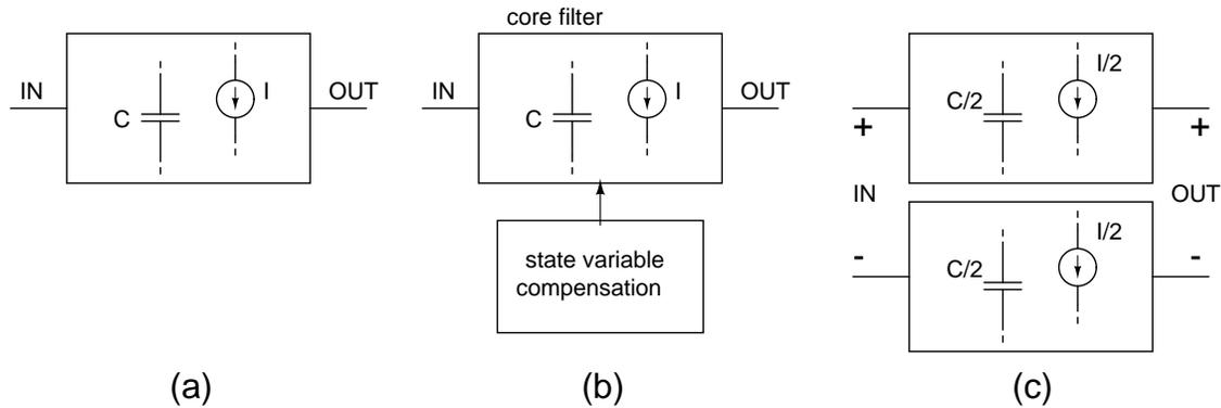
Figure 3.5: (a) Class-A single ended log-domain filter, (b) Dynamic biasing as in section 2.2.3, (c) Dynamic biasing as in section 3.2.
