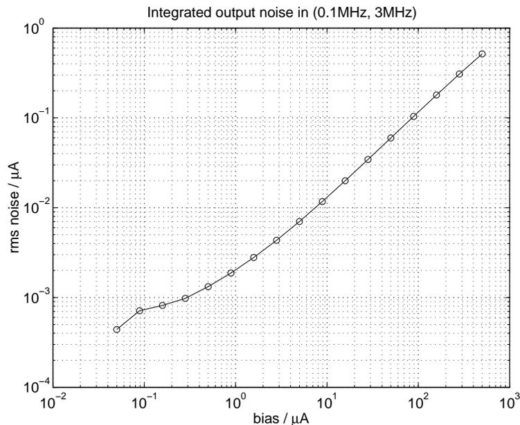
Figure 7.14: Output noise integrated in 100 kHz to 3MHz band.
