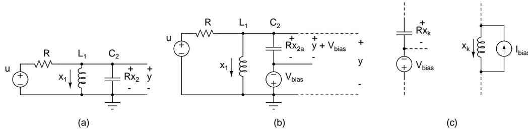
Figure 2.11: (a) RLC Bandpass filter, (b) Modification to ensure positive quiescent state variable  $x_2$ , (c) General modification to ensure positive quiescent state variables  $x_k$ .
