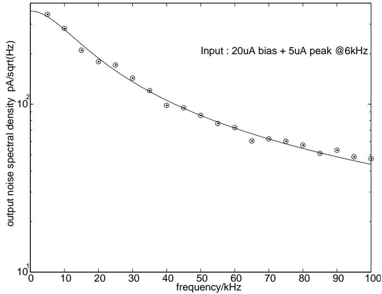
Figure 6.13: Output noise of a first order class-A filter—lines: calculated, circles: measured.
