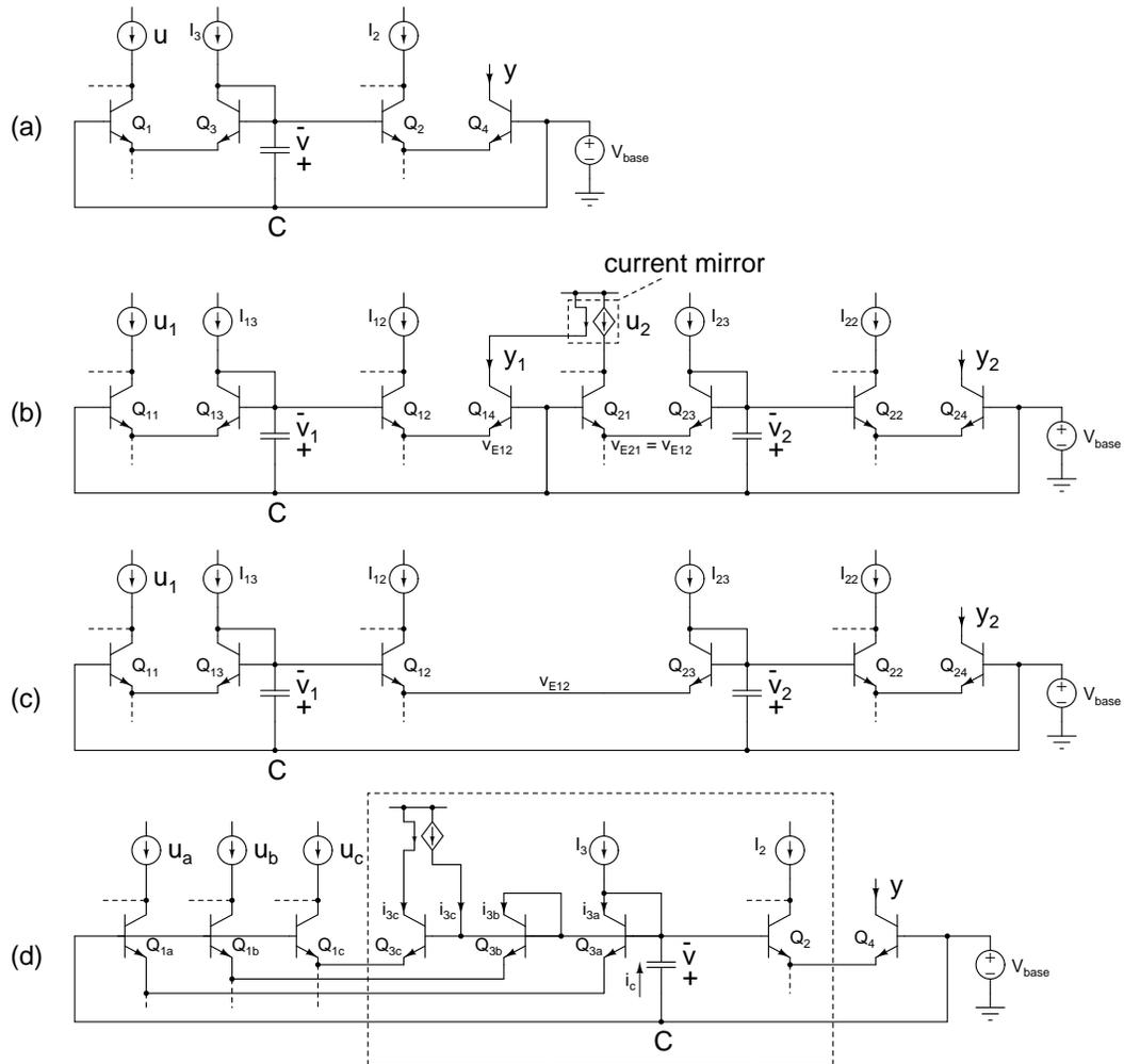
Figure 7.2: (a) First order log-domain filter in Fig. 2.16, (b) Cascading two stages, (c) Eliminating redundancies in (b), (d) Modification to accept multiple inputs with positive and negative weights.
