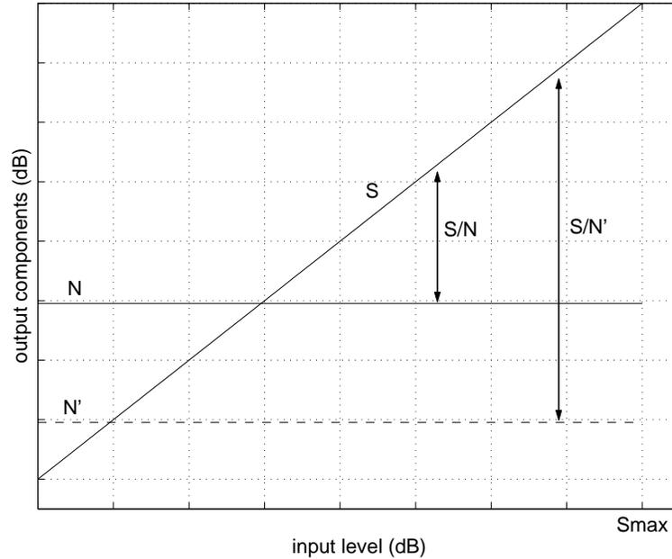
Figure 2.2: Output signal and noise in a typical active filter.
