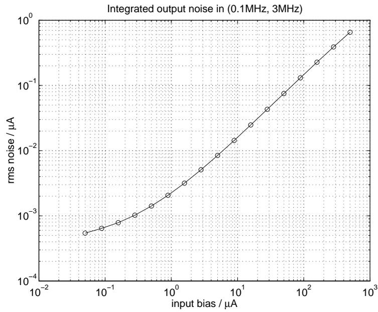
Figure 7.25: Output noise integrated in the 100 kHz to 3MHz band.
