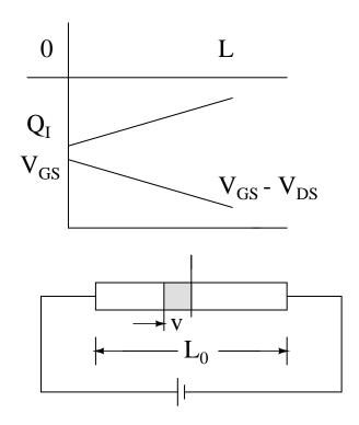
Gate to channel voltage is smaller at Drain than at Source.
