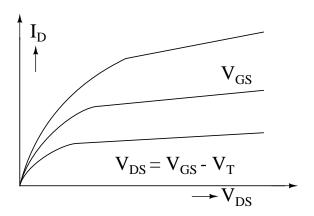
$$I_{D} = \mu_{n} C_{ox}(\frac{W}{L})((V_{GS} - V_{T})V_{DS} - \frac{V_{DS}^{2}}{2}) \qquad 0 \le V_{DS} \le V_{GS} - V_{T}$$
