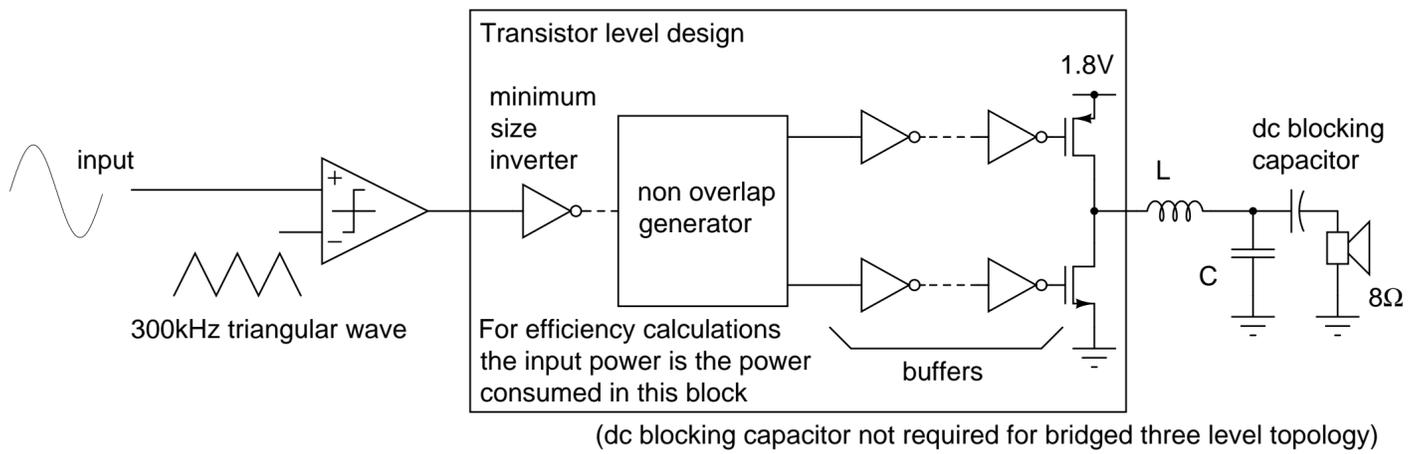
(a) Open loop half bridge class D amplifier
