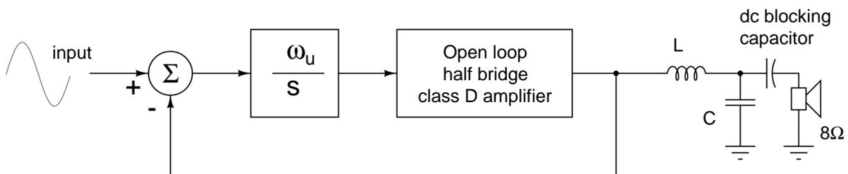
(b) Closed loop half bridge class D amplifier
