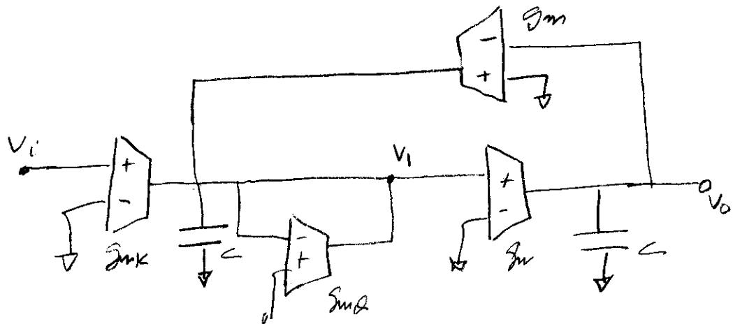
$$\frac{V_o}{V_i} = \frac{g_{m1}}{g_m} \frac{\frac{1}{(sC/g_m)^2 + \frac{sC}{g_m g_{m2}} + 1}}{}$$
