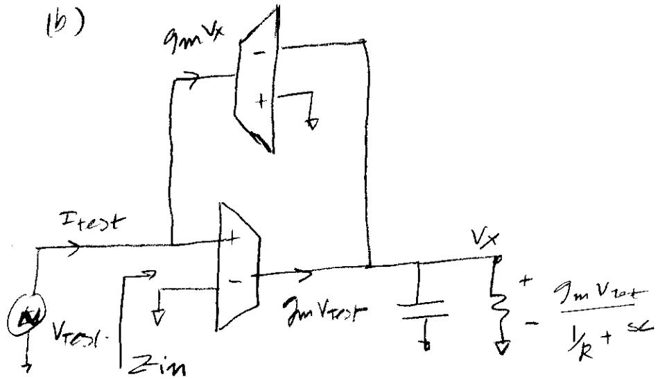
$$V_x = (g_m V_{TEST}) \left[ \frac{1}{Y_R + SC} \right]$$
