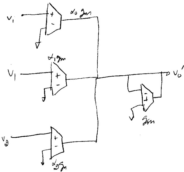
$$\frac{V_0'(s)}{V_1'(s)} = \frac{(\alpha_0 + k\alpha_2) + (\alpha_0 + \alpha_1 k\theta) \frac{s}{\omega_{np}} + \alpha_0 \left( \frac{s}{\omega_{np}} \right)^2}{1 + \frac{s}{\omega_{np}} + \left( \frac{s}{\omega_{np}} \right)^2}$$
