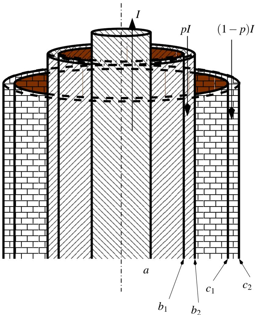
We have three coaxial cylinders. The inner one is hollow, and the middle and outer ones are hollow. All the solid portions have a conductivity  $\sigma$  and the gaps are air-filled.
