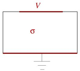
The material has a conductivity  $\sigma$  and its top lead extends from -a < x < a, while the device extends from -L < x < L. The device is *d* metres in height along  $\hat{y}$ . The problem is to find the current that is injected.
