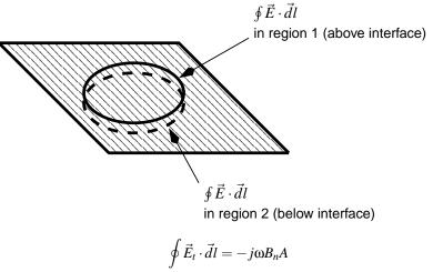
where A is the area of the loop. Since the tangential Electric Field is continuous, the loop integral is the same on both sides of the interface. Which means that  $B_n$  must also be continuous.
