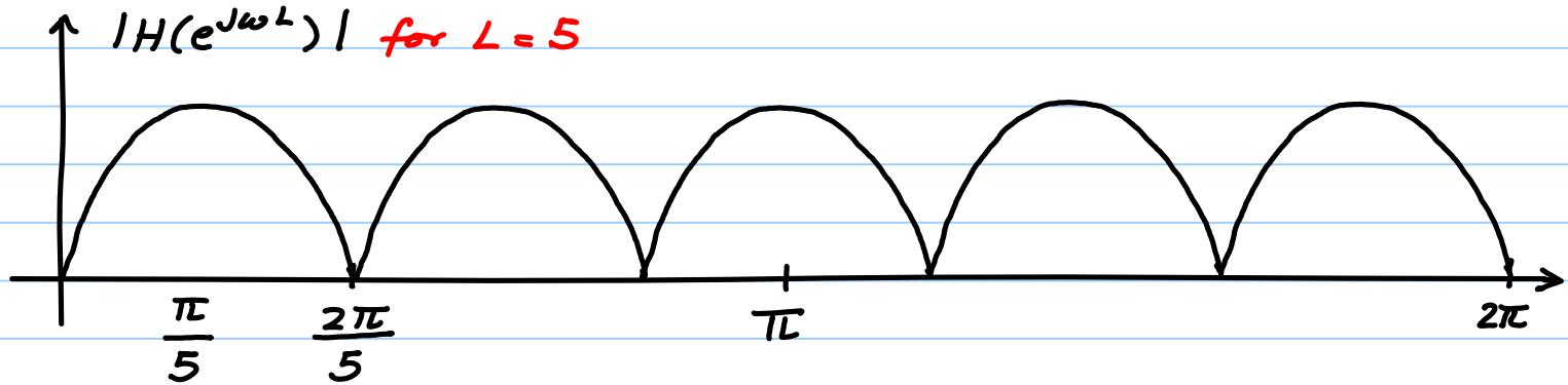
$$\text{If } H(z) = \frac{1}{N} \frac{1-z^{-N}}{1-z^{-1}}, \text{ then } |H(e^{j\omega})| = \left| \frac{\sin N\omega/2}{\sin \omega/2} \right|$$
