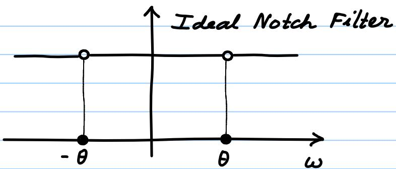
The given notch filter's response can be improved by adding poles at  $r e^{\pm j\theta}$  where  $r$  is close to 1.
