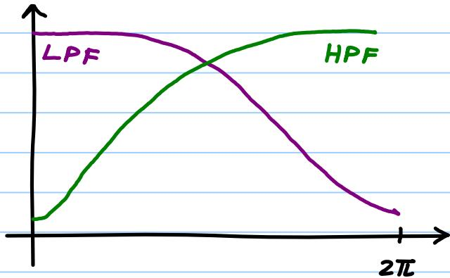
Lowpass and Highpass filters realized using single complex pole:
