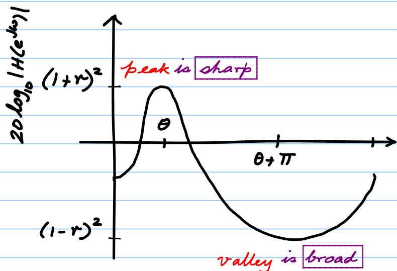
Pole near the unit circle **boosts** the frequency response
