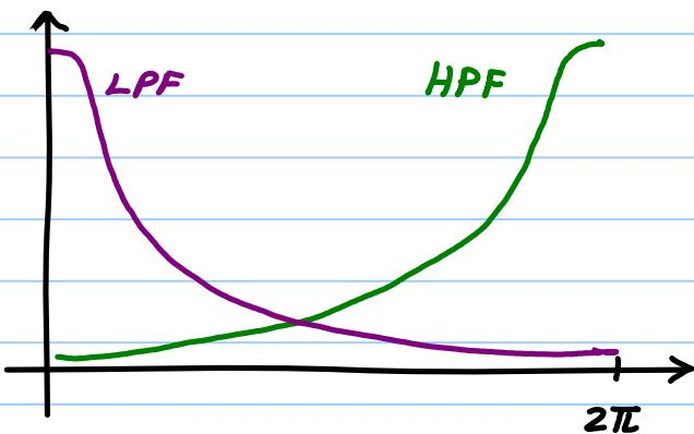
The main difference between an LPF realized using a pole versus another realized using a zero is the narrowness of the passband.
