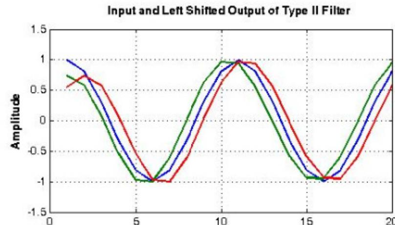
Neither of the integer shifts closest to  $0.5 \times (N-1)$  produces exact alignment with the input
