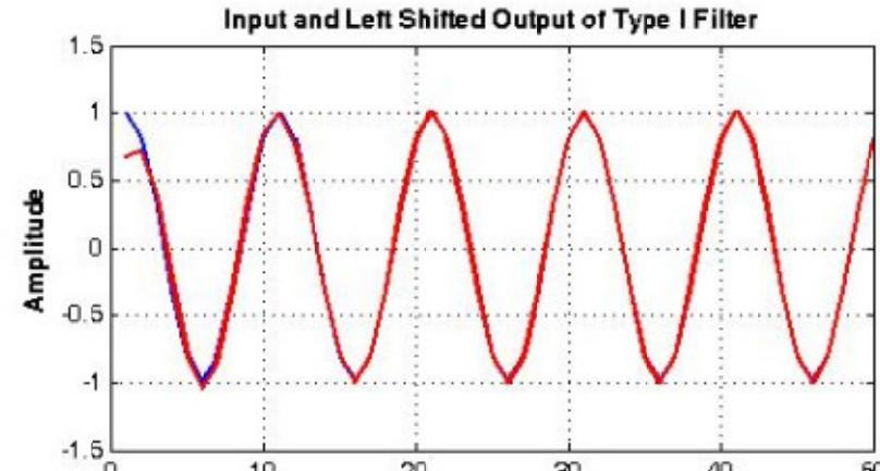
Integer shift equal to  $0.5 \times (N-1)$  produces exact alignment with the input
