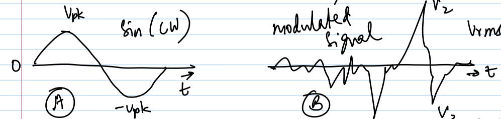
& PA should not clip @  $v_1, v_2, v_3$  etc.
