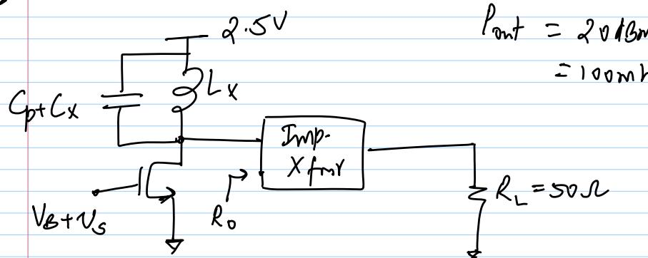
Assume  $V_{o,\min} = V_{DSAT} + V_{margin}$
