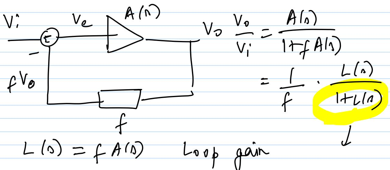
$|L| \geq 1$ ,  $\underline{\angle} = -180^\circ$   $\Rightarrow$  oscillations
