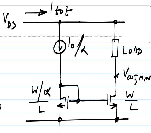
① The current mirror shown on the right delivers a current  $I_o$  to the load. The reference branch current can be tailored using the parameter  $\alpha$ .
