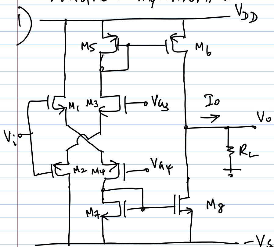
\*  $V_{GS3}$  &  $V_{GS4}$  determine class B/AB mode
