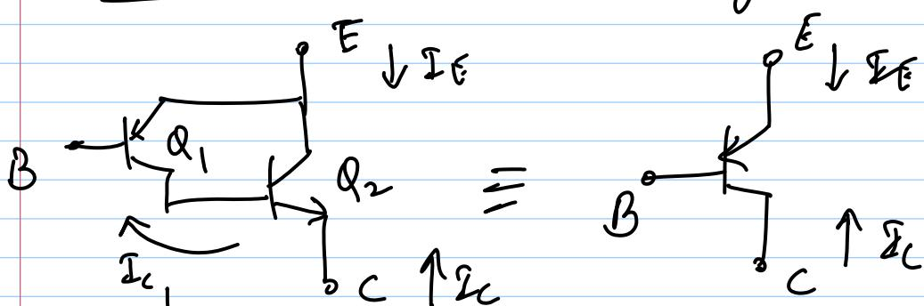
$$I_{C_1} = -I_S \exp\left(-\frac{V_{BE}}{V_T}\right)$$
