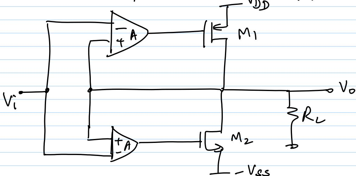
\* Error amps drive  $V_i = V_o$  (-ve f.b.)
