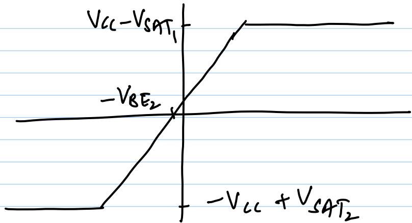
\* V<sub>AB</sub> = constant  $\Rightarrow |\Delta V_{BE1}| = |\Delta V_{BE2}|$
