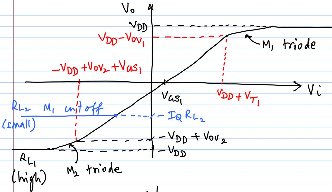
slope @  $V_i/V_o = 0$  point = incremental gain
