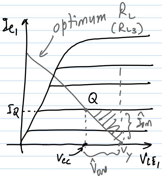
$$V_x = V_{CC} + I_Q R_{L2}$$
