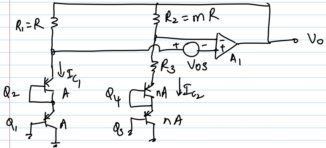
$$R_2 = m R_1 \Rightarrow I_{C_1} \approx m I_{C_2}$$
