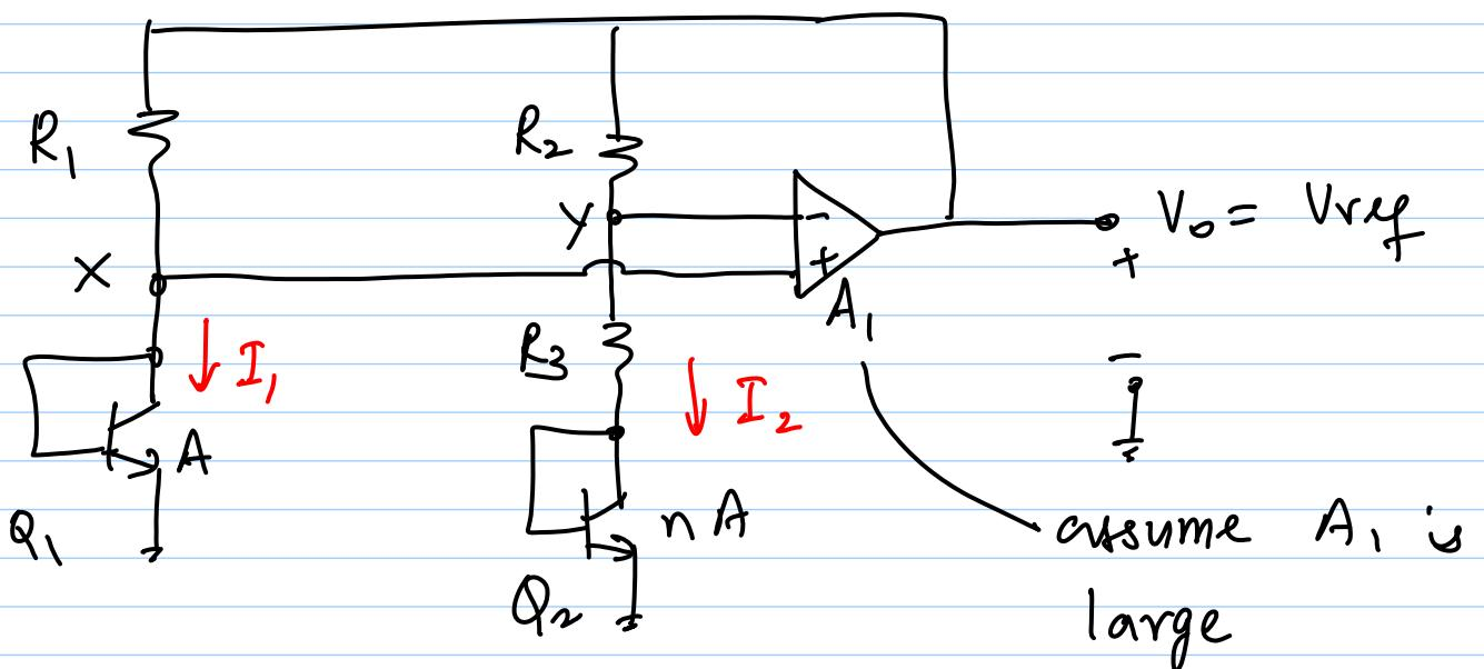
$$\Rightarrow V_x = V_y \text{ (due to f.b. loop)}$$
