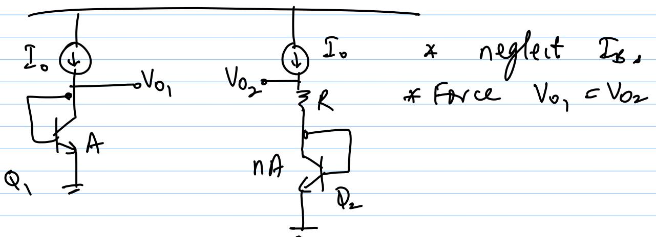
$$V_{BE_1} = I_0 R + V_{BE_2}$$
