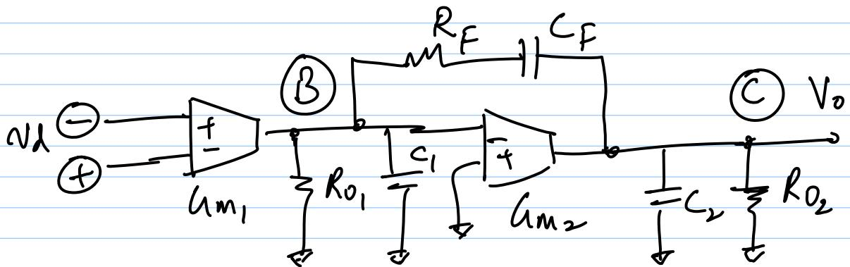
Basic idea: @ high freq., develop a small-signal voltage across  $R_F$  that cancels small-signal voltage @ output
