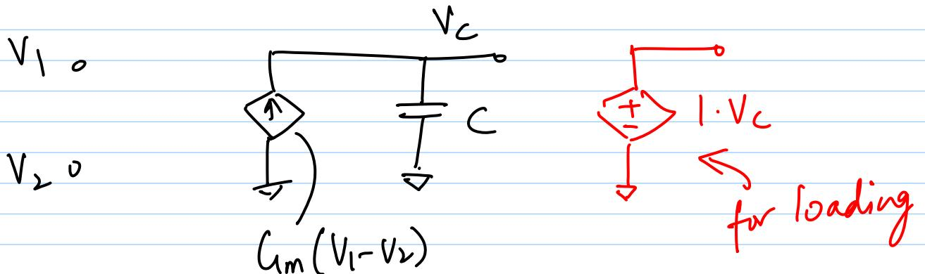
$$V_c = \frac{G_m}{C} \int (V_1 - V_2) dt$$
