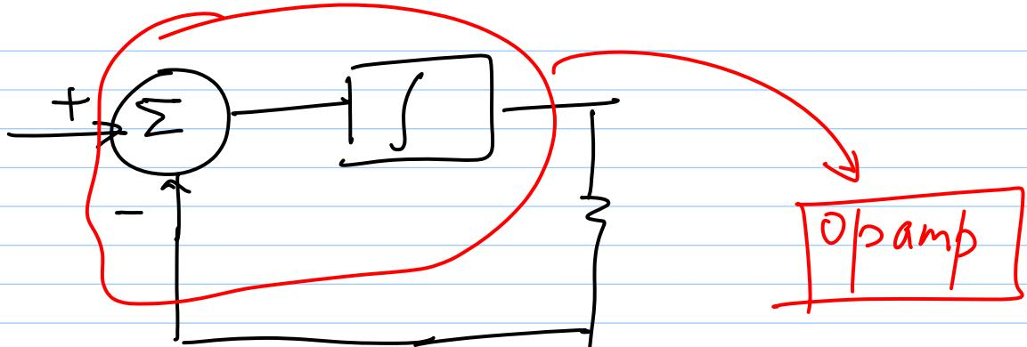
$$V_1 \quad \text{---} \quad \left[ \begin{array}{|c|} \hline \text{ } \\ \hline \end{array} \right] \quad \text{---} \quad \omega_u \int (V_1 - V_2) dt$$
