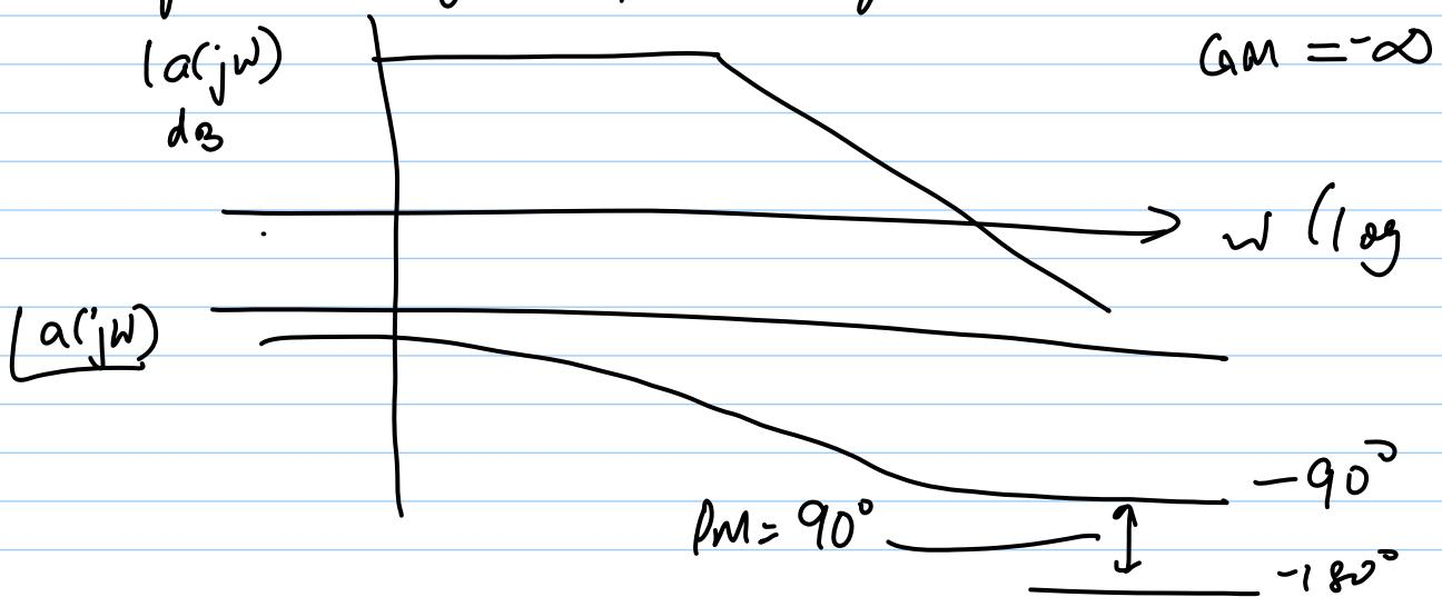
typical  $P_M \sim 60^\circ$  (lower limit of  $45^\circ$ )
