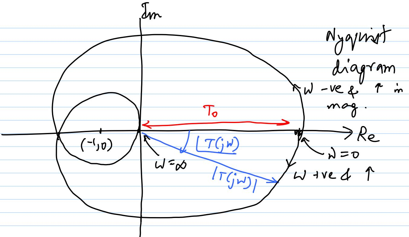
$$\omega = 0 \Rightarrow T(j\omega) = T_0, \quad \underline{\text{[ } T \text{ ]}} = 0$$
