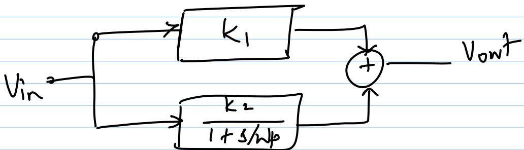
$$V_{out}(\lambda) = k_1 V_{in}(\lambda) + \frac{k_2}{1 + s/w_p} V_{in}(\lambda)$$
