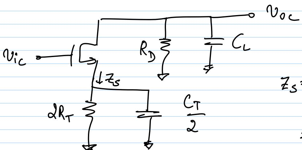
$$Z_s = \frac{2R_T / (\delta C_T / 2)}{2R_T + \frac{2}{\delta C_T}} = \frac{2R_T}{1 + \delta C_T R_T}$$
