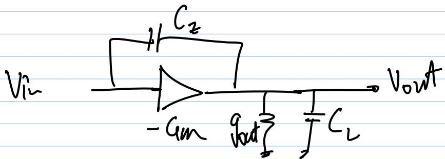
$$V_{out} = i_{out} Z_{out}$$
