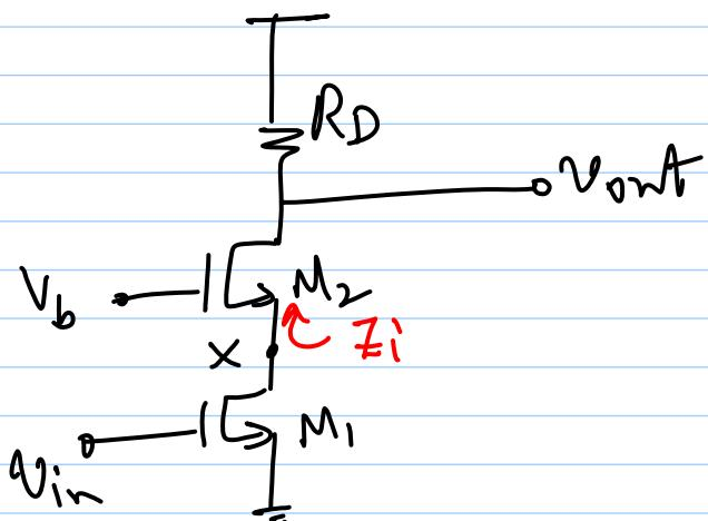
$$\frac{V_{out}}{V_{in}} \approx -g_m R_D$$
