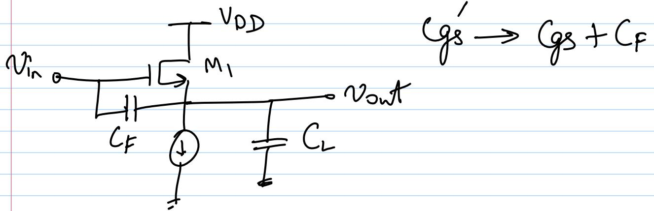
$$\omega_p = -\frac{(g_m + g_{mbs} + g_{ds})}{C_{gs} + C_F + C_{sb} + C_L}$$
