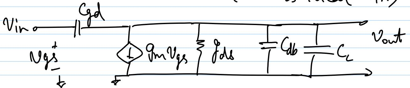
$$H(s) = \frac{V_{out}(s)}{V_{in}(s)}$$
