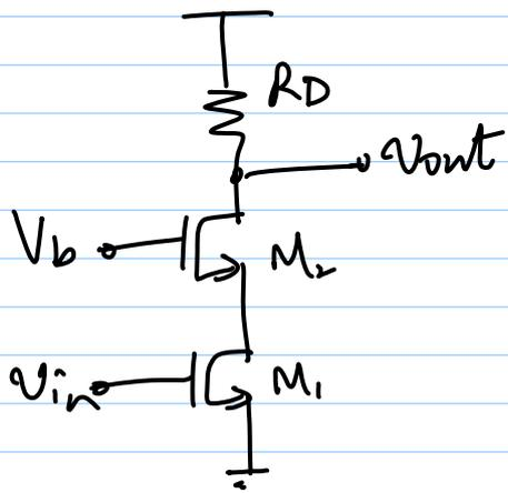
$$\frac{\overline{v_{n,out}^2}}{\Delta f}(M_1, R_D) = \left[ 4KTg_D + 4KT\gamma_1 g_{m1} \right] R_D^2$$
