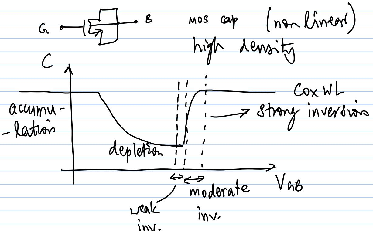
typically  $C_{MOS} \sim 2-3 \times C_{MOM}$  for given area
