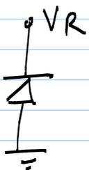
$$C_{\text{var}} = \frac{C_0}{\left(1 + \frac{V_R}{\phi_B}\right)^m}$$
