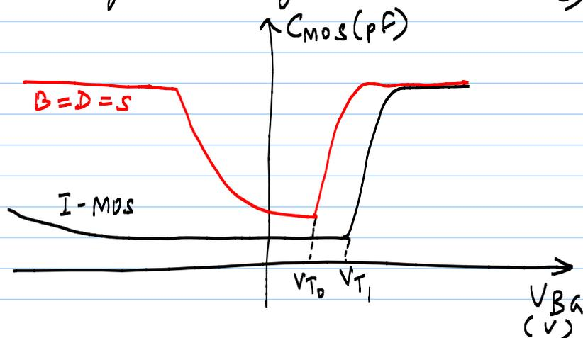
\*  $V_{T1} > V_{T0}$  due to substrate effect ( $V_B > V_S$ )
