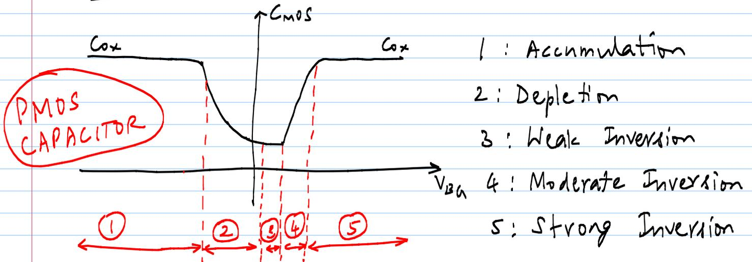
$V_{BG} \gg |V_{T1}| \Rightarrow$  strong inversion (transistor behaviour)
