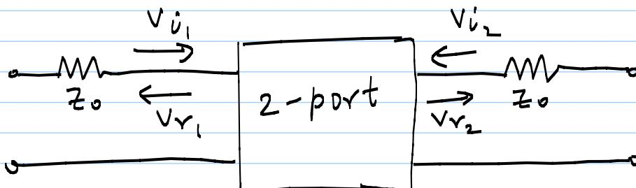
$$\begin{bmatrix} V_{r1} \\ V_{r2} \end{bmatrix} = \begin{bmatrix} S_{11} & S_{12} \\ S_{21} & S_{22} \end{bmatrix} \begin{bmatrix} V_{i1} \\ V_{i2} \end{bmatrix}$$
