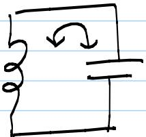
$$V_{\text{out}, \text{pk}} = I_{\text{pk}} \cdot R \Rightarrow E_{\text{tot.}} = \frac{1}{2} C (I_{\text{pk}} \cdot R)^2$$
