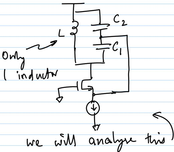
$$\omega_0 = \frac{1}{\sqrt{L - \frac{C_1 C_2}{C_1 + C_2}}}$$
