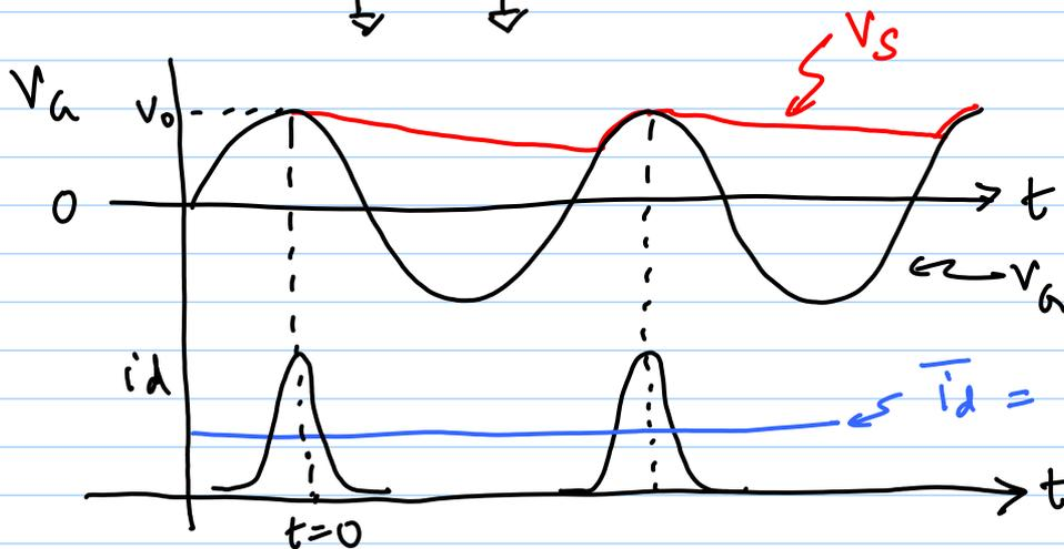
\*  $M_1$  conducts only when  $V_a$  is large ( $\sim V_0$ )
