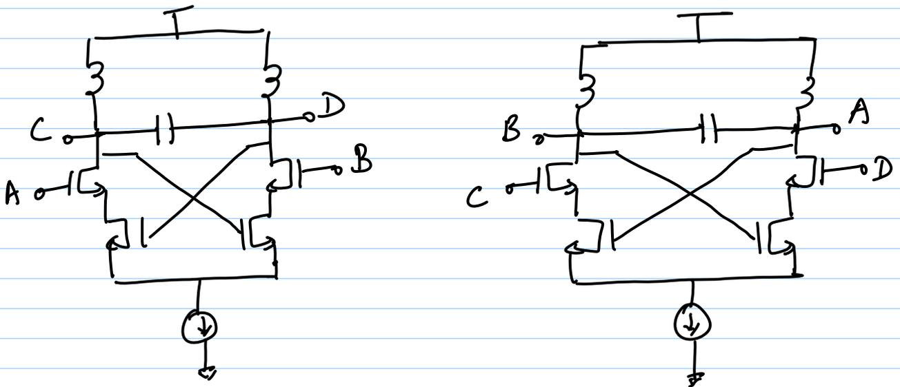
\* (a) & (b) : extra parasitic cap on tank ( $\downarrow$  tuning range)
