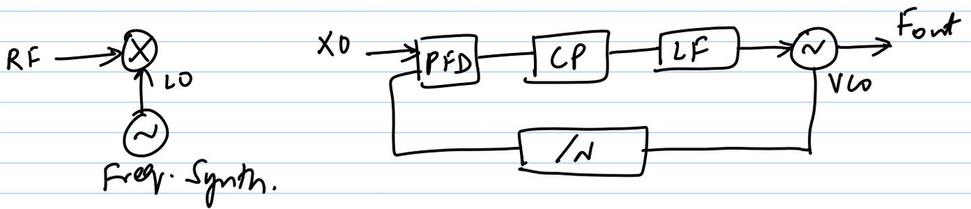
\* Autonomous ckt (i.e. needs to be locked with a PLL)
