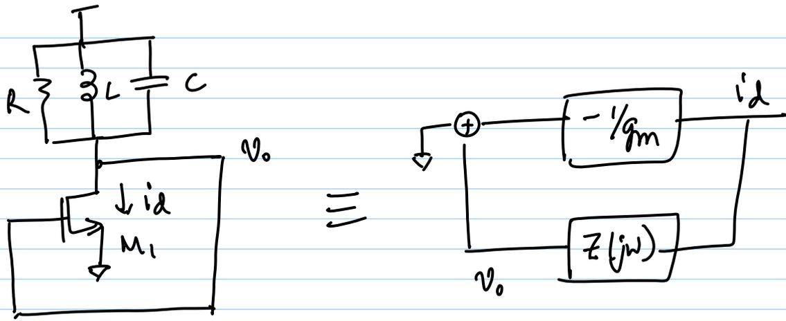
(a) resonance, RLC tank phase shift = 0
