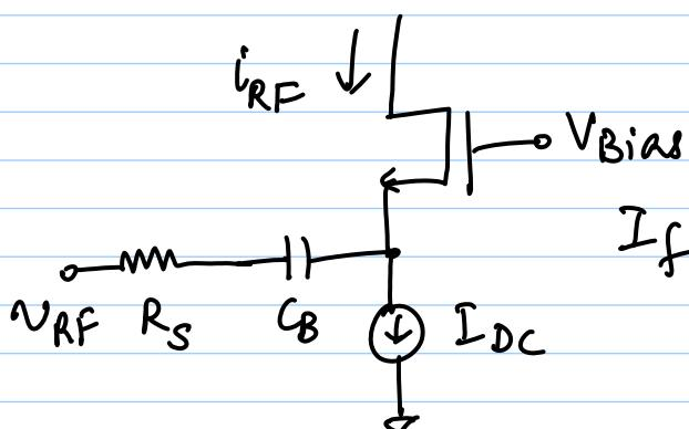
$$g_{m,\text{eff.}} = \frac{g_m}{1 + g_m R_s + s R_s C_{gs}}$$
