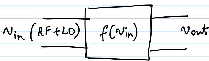
$$v_{\text{out}} = \sum_{n=0}^N c_n (v_{\text{in}})^n$$
