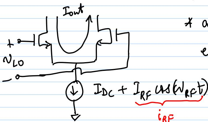
\* assume  $V_{LO}$  is large enough to switch currents completely between two sides.
