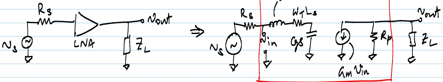
$$G_T = \frac{\text{Power delivered to load}}{\text{Power available from source (max)}} = \frac{P_{\text{load}}}{P_{\text{available,source}}}$$
