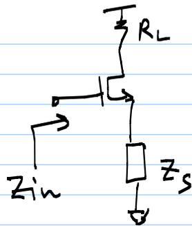
\* assume transistor model with only  $C_{gs}$  &  $g_m$
