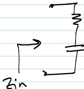
$$\frac{C_{gs}}{1 + g_m R_s} \approx \frac{1}{\omega_T R_s}$$
