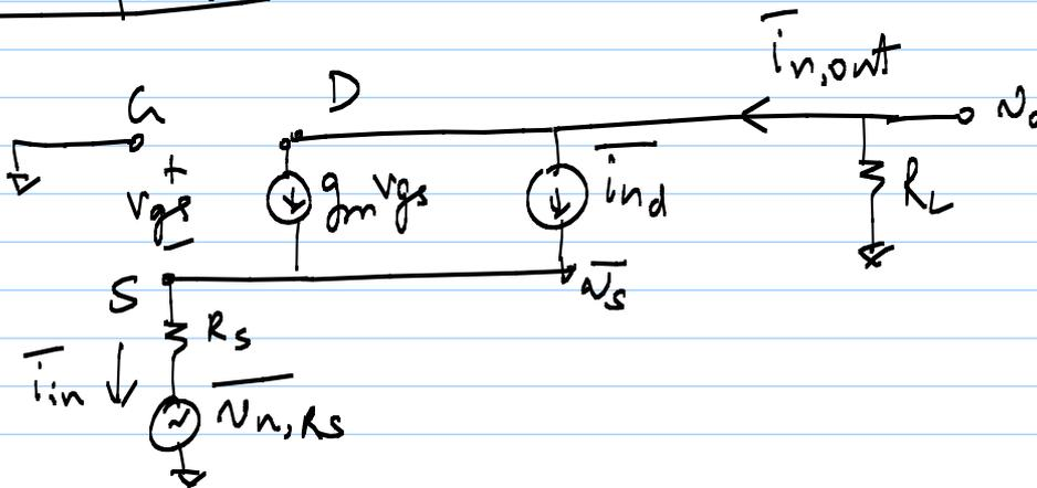
\*  $\overline{i_{ind}}$  and  $\overline{v_{n,R_s}}$  are uncorrelated
