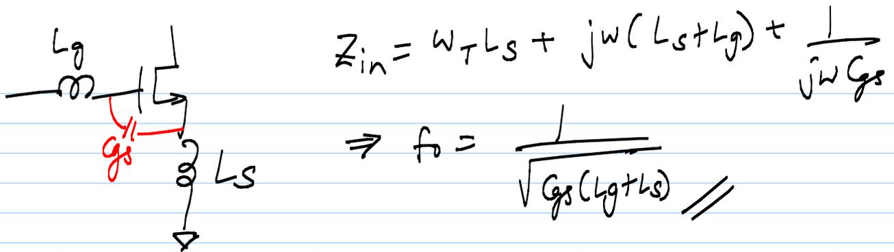
$$Z_{in} = \omega_T L_S + j\omega(L_S + L_g) + \frac{1}{j\omega C_{gs}}$$
