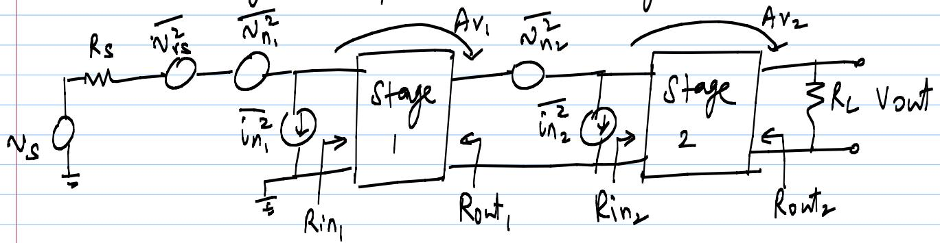
$A_{V1}, A_{V2} \rightarrow$  unloaded voltage gains of stage 1 & 2
