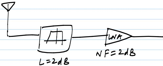
$$F_{tot.} = F_{filt.} + \frac{F_{LNA}-1}{L^{-1}} = L + L \cdot (F_{LNA}-1)$$
