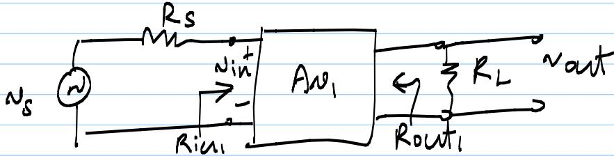
$$R_s = R_{in1}; R_{out1} = R_L$$
