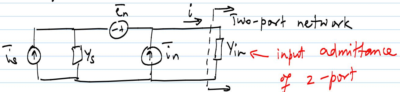
$$i_s = i_n \cdot \left( \frac{Y_{in}}{Y_s + Y_{in}} \right) + (i_n + e_n Y_s) \cdot \left( \frac{Y_{in}}{Y_{in} + Y_s} \right)$$
