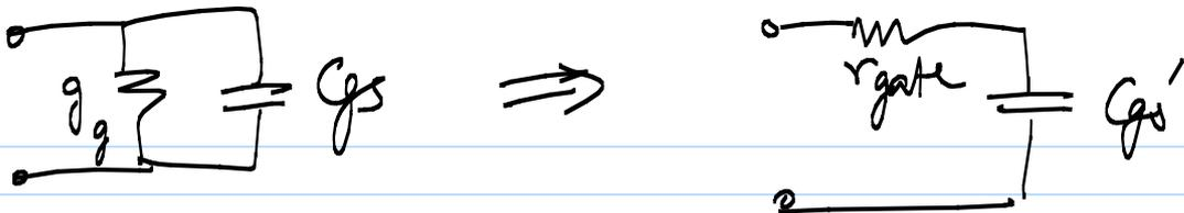
\*  $C_{gs}' \approx C_{gs}$  (assume high Q)  $\left\{ C_{gs}' = C_{gs} \cdot \frac{1+Q^2}{Q^2} \right\}$
