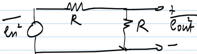
$$\left. \begin{array}{l} \text{Noise power delivered to} \\ \text{load resistor in a 1Hz BW} \end{array} \right\} = \frac{(\overline{e_n}/2)^2}{R} = \frac{\overline{e_n^2}}{4R} \text{ (W/Hz)}$$
