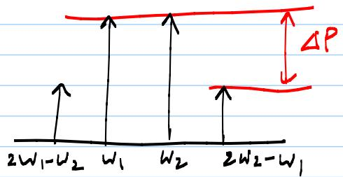
$$|IP_3|_{dBm} = \frac{\Delta P_{dB}}{2} + |Pin|_{dBm}$$
