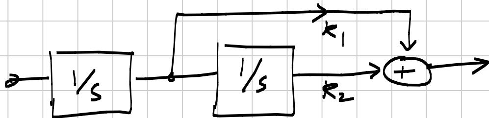
Determine  $k_1$  &  $k_2$  so that the NTF is  $(1 - z^{-1})^2$  for the following DAC pulses
