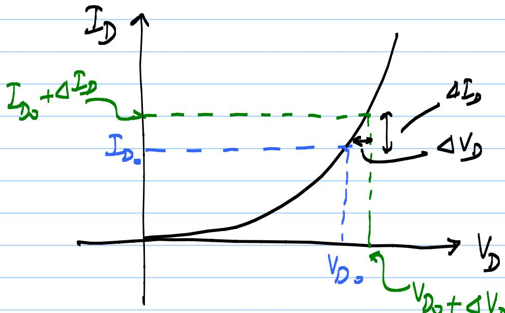
$$\frac{\Delta I_D}{\Delta V_D} = \left. \frac{d I_D}{d V_D} \right|_{(I_{D_0}, V_{D_0})}$$
