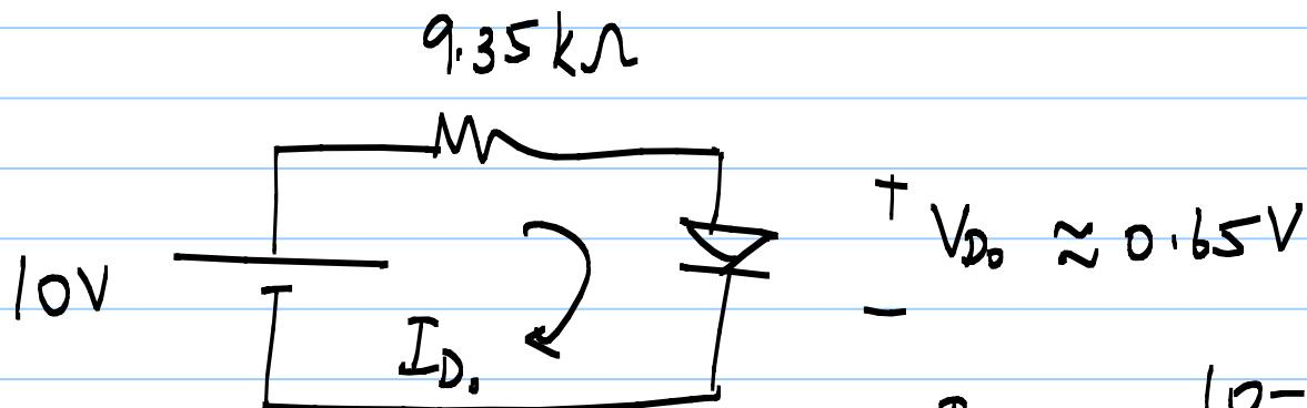
$$I_{D_0} = \frac{10 - 0.65}{9.35\text{ k}\Omega} = 1\text{ mA}$$
