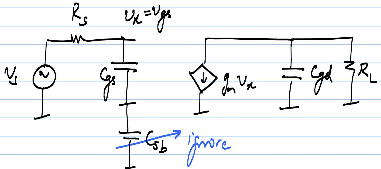
$$v_x(s) = \frac{1/s C_{gs}}{R_s + 1/s C_{gs}} \cdot v_s(s)$$
