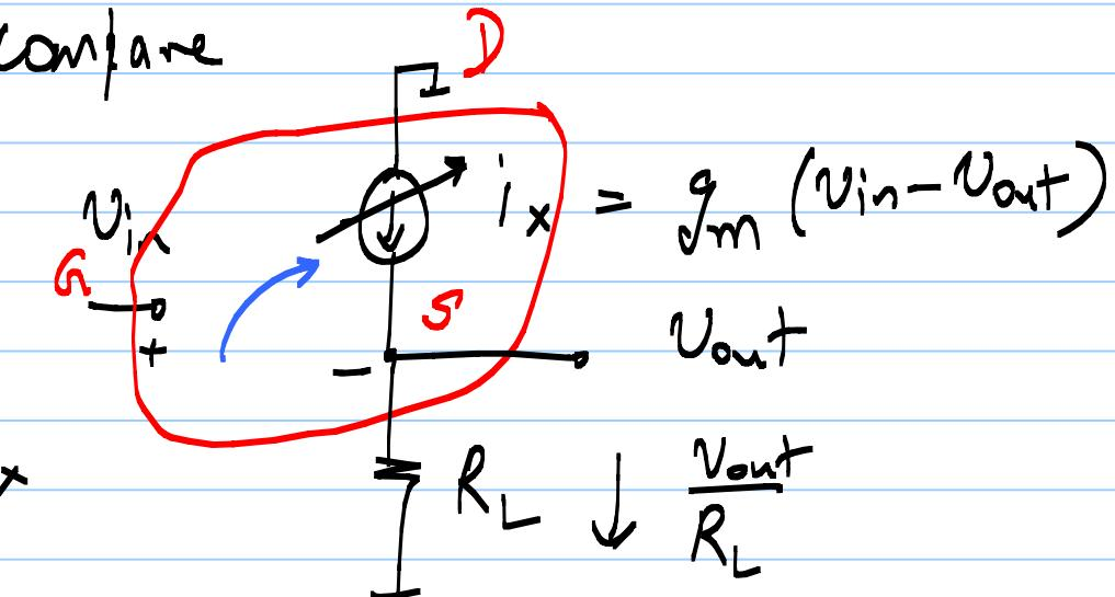
output current  $\frac{V_{out}}{R_L} = g_m(V_{in} - V_{out})$  if in neg. f.b.
